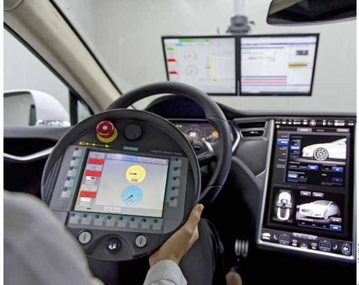
Test situation inside the vehicle to be tested, with a Simatic Mobile Panel
