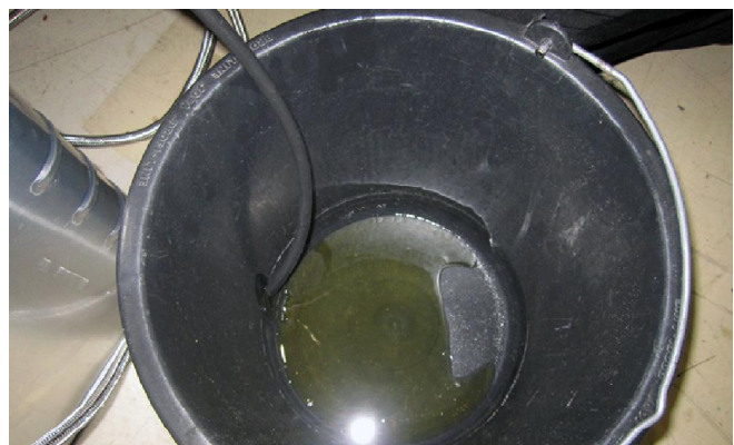
2.4. Connect the second reinforced tubing to the bottom sampling kit valve and from the other side with the black tygon flexible tubing with a coupling connector. The other end of the black flexible tubing leads to the oil disposal vessel. Open the red stop cock. Use this set up to rinse approx. 3 l of oil.
