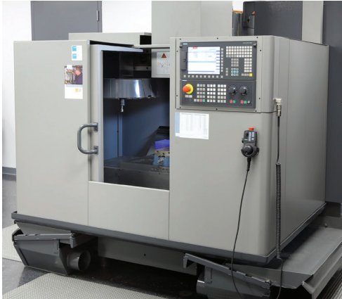
After completion of the machine retrofit with SINUMERIK 828D
