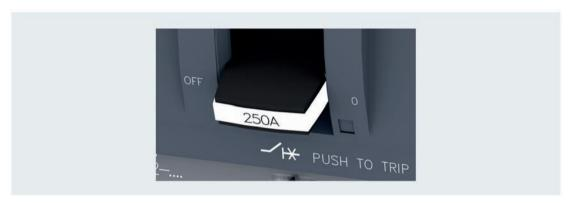
With its wide surface area, the ergonomic handle is designed to assist manual operation of the circuit breaker. The white strip around the edge of the handle makes it easy to identify in conditions of poor visibility. The additional rated operational current information stamped on the white strip also significantly eases identification of the circuit breaker when it is one of many breakers in a large switchboard installation.
