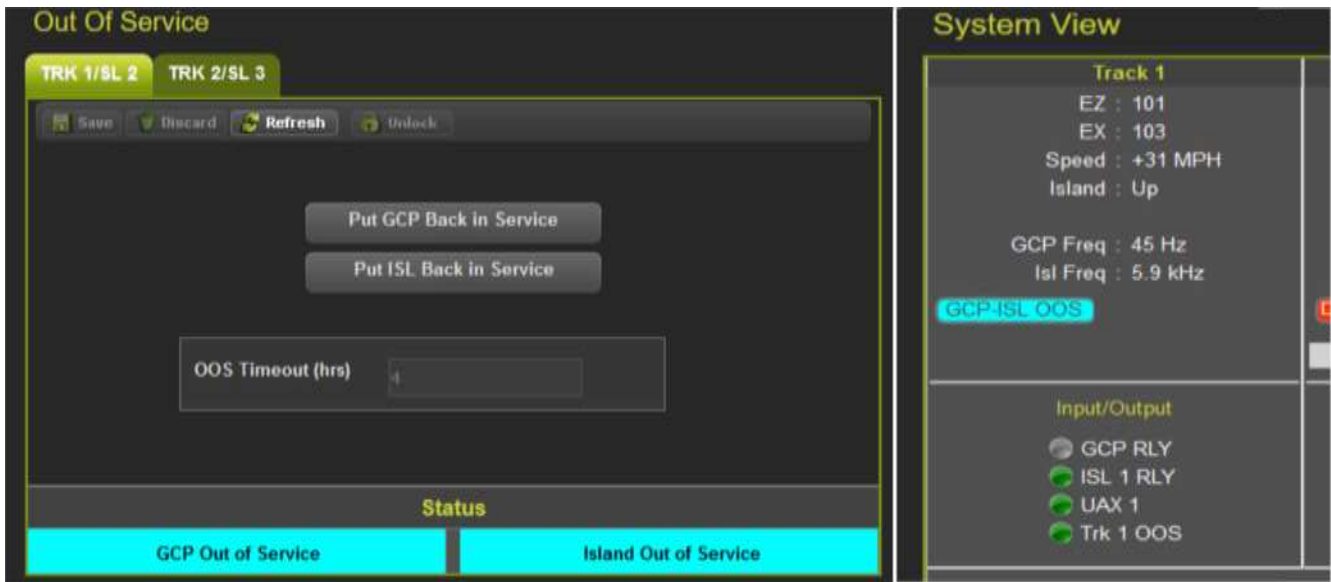
Figure 4-137 Island Out of Service Indications on WebUI
