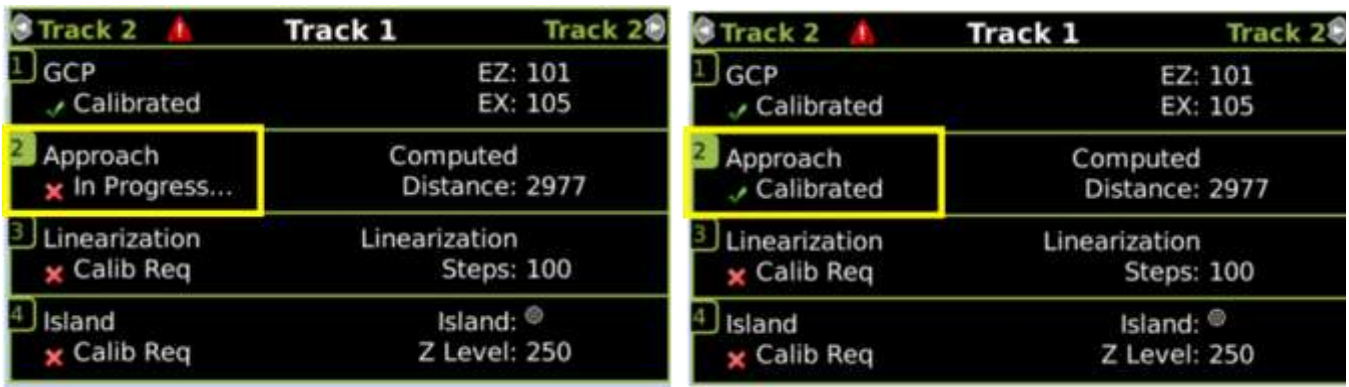
Figure 6-7 GCP Approach Calibration Window Before and After Approach Calibration
