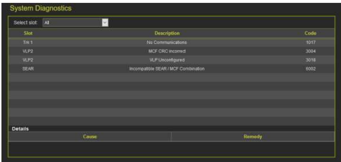
Figure 4-174 WebUI System Diagnostics when VLP is Unconfigured due to MCF CRC Error
