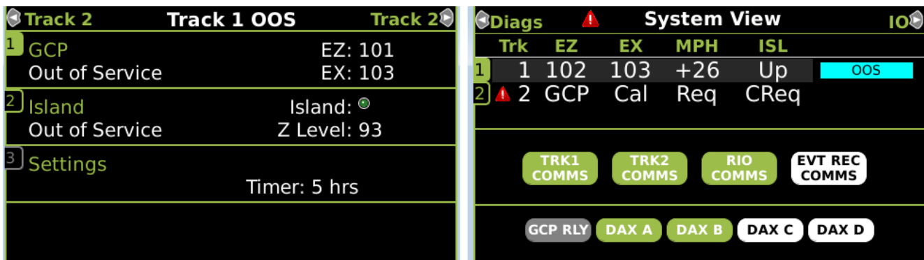
Figure 7-30 Island Out of Service Indications on Display
