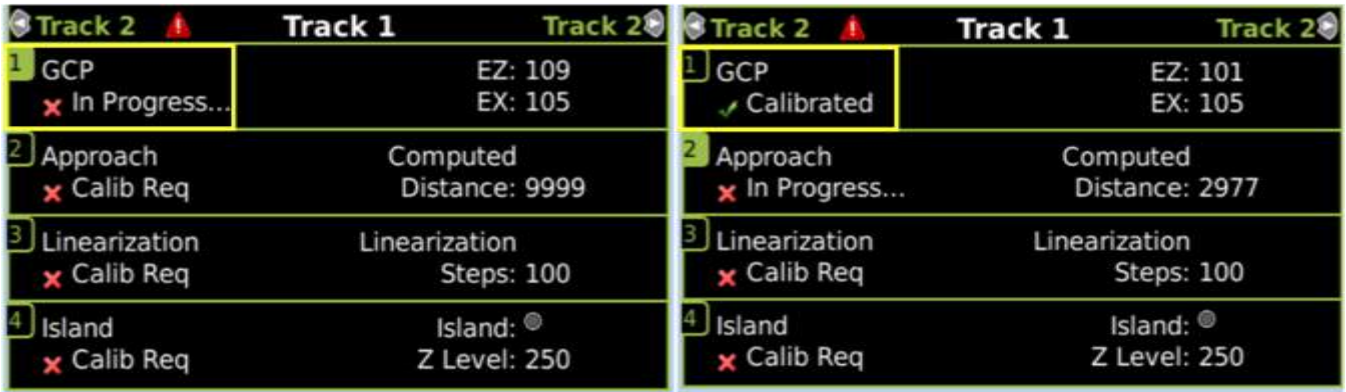
Figure 6-5 Calibration In Progress and Complete
