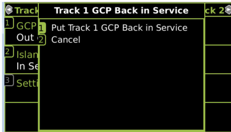
Figure 4-30 Placing a Track Back in Service
