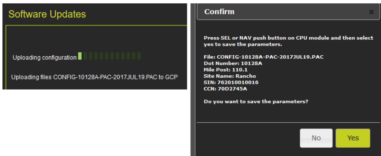
Figure 4-162 WebUI: Configuration Upload Progress and Final Check
