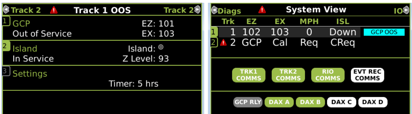
Figure 7-27 Out of Service Indications on Display
