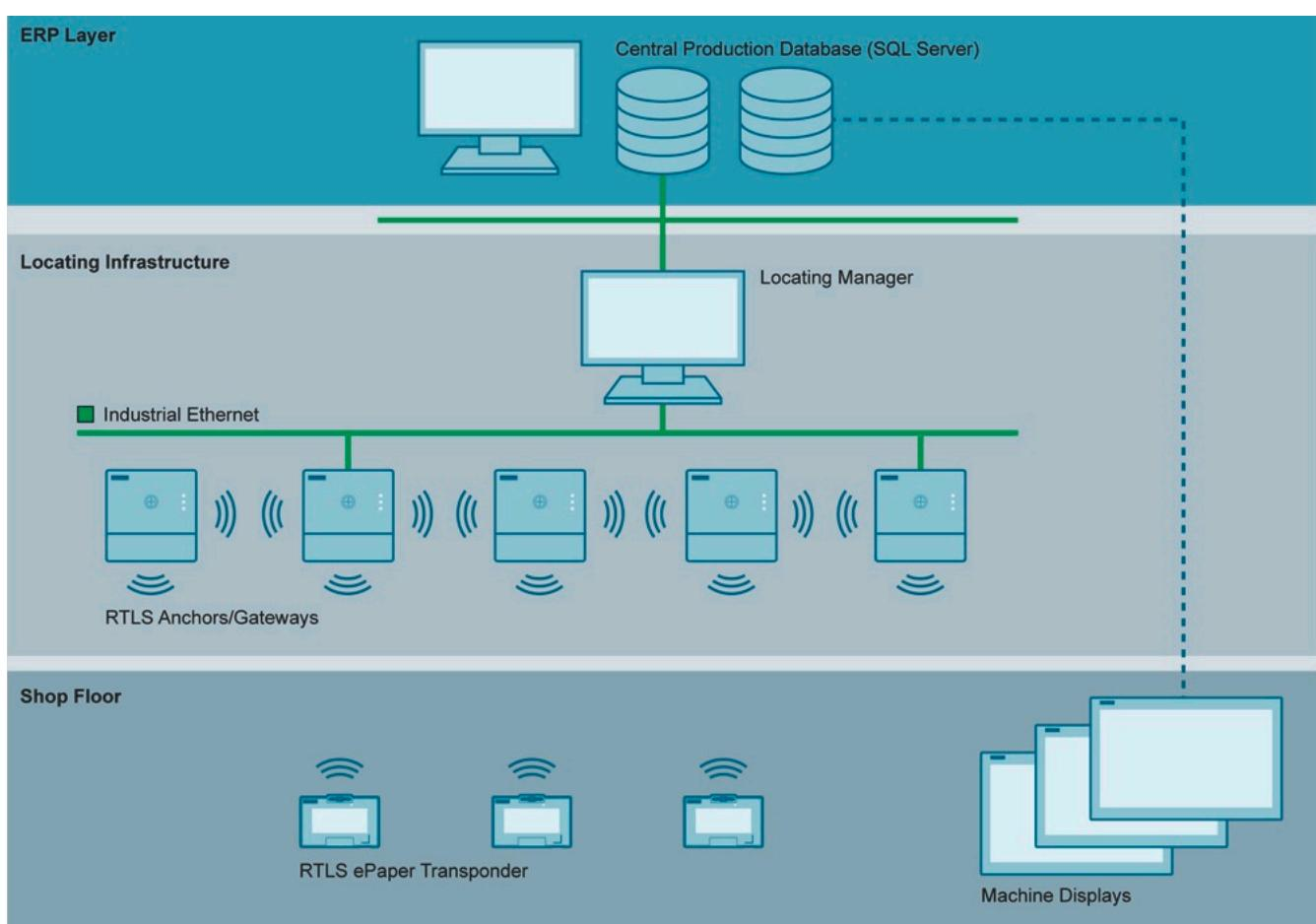
The SQL interface of the SIMATIC RTLS Locating Manager allows for easy, high-performance integration with the ERP system at Materials Solutions.
