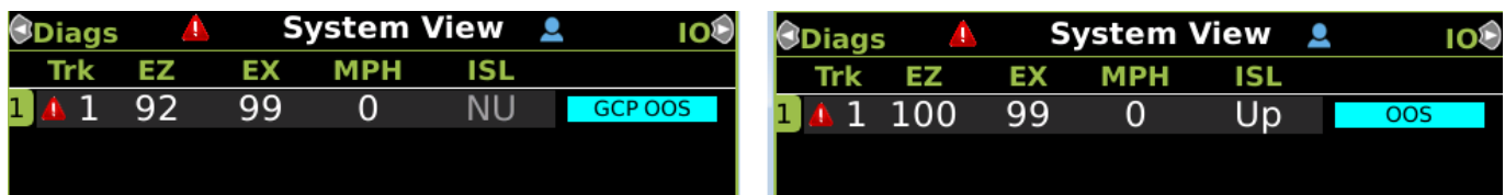
Figure 3-4 System View Out Service Indication
