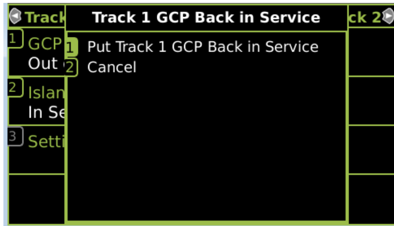
Figure 3-20 Placing a Track Back in Service
