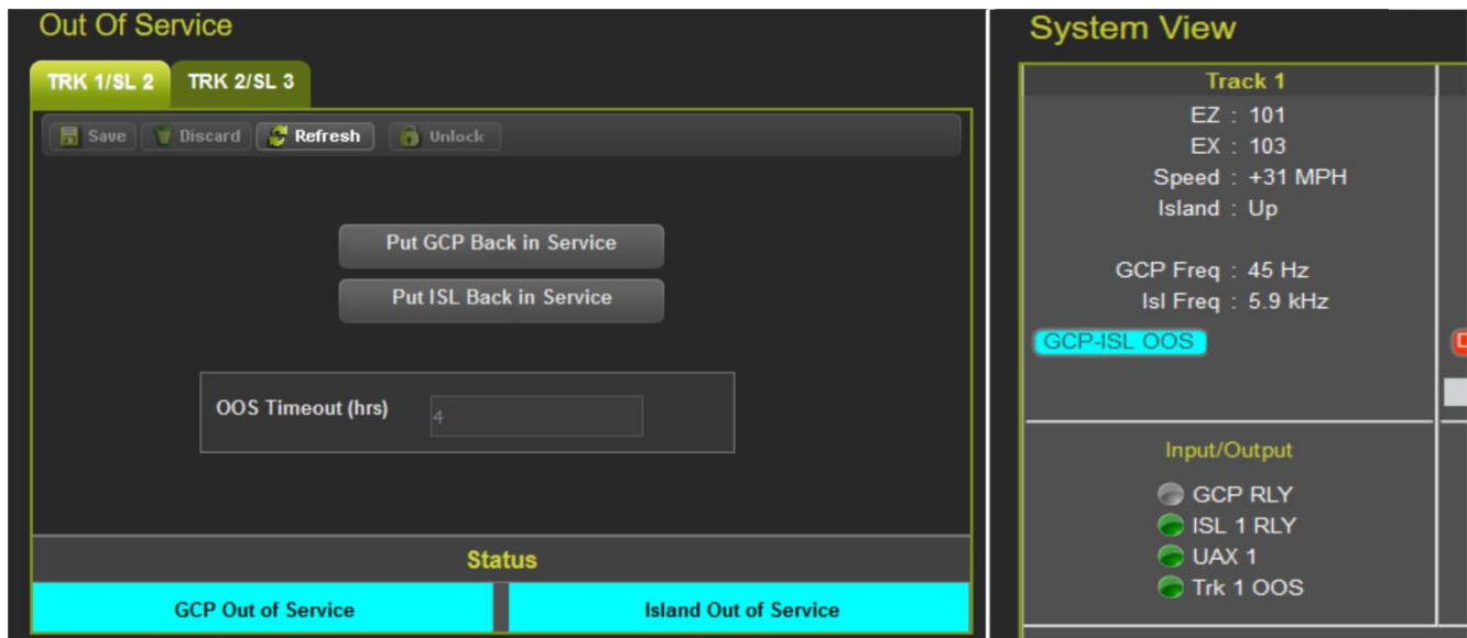
Figure 3-58 Island Out of Service Indications on Web UI
