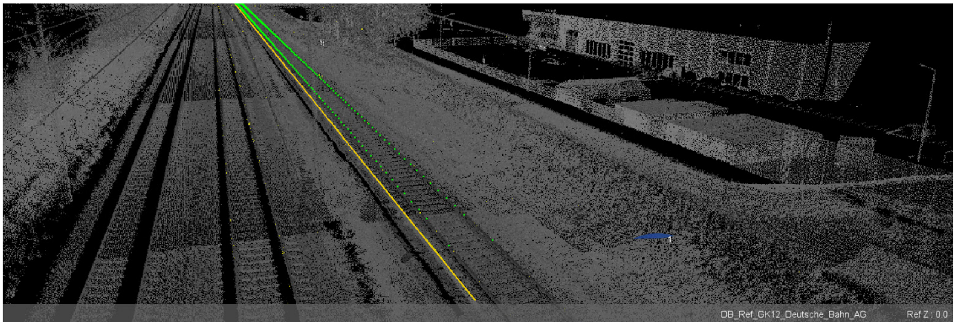
Scaled double line track layout (SDTL) with georeferenced wayside track elements
