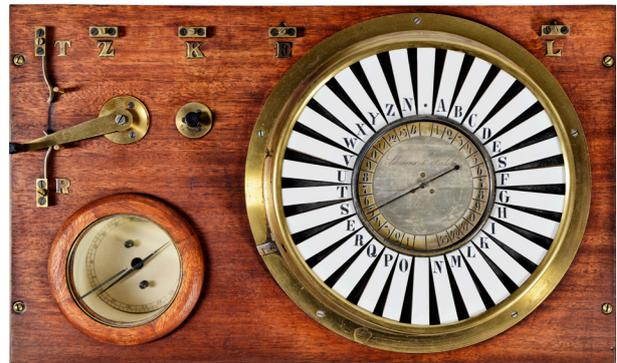
Werner von Siemens laid the cornerstone of the "Telegraphen-Bauanstalt von Siemens & Halske" with the invention of the pointer telegraph.
