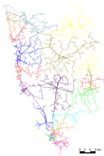
Figure 1: Distribution network of Elektroistra Pula region focused in the automation study.
