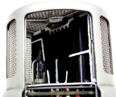
Image left: R5 optical smoke detector. The unit has been cut open to illustrate its internal components.
