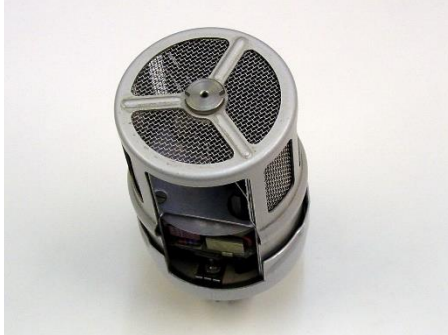
Image left: R5 optical smoke detector. The unit has been cut open to illustrate its internal components.
