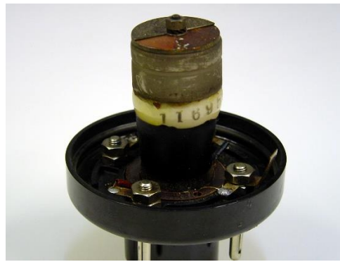
Right image: The core component of the F1, still visible in this photo, was a unit consisting of a cold cathode tube and a reference ionization chamber.
