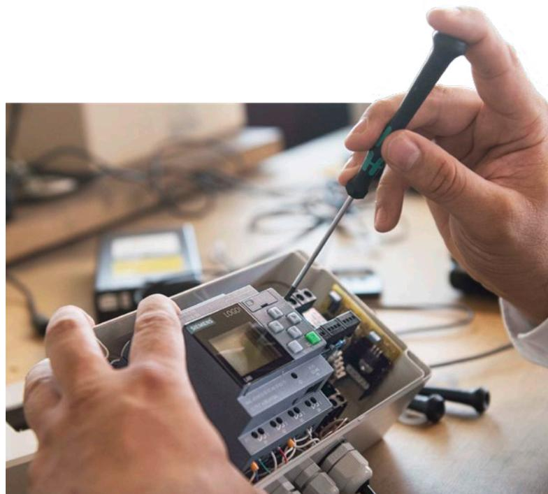
In addition to defined movements, the logic module also controls the electrical lift systems' various safety functions for TVs, monitors and projectors
