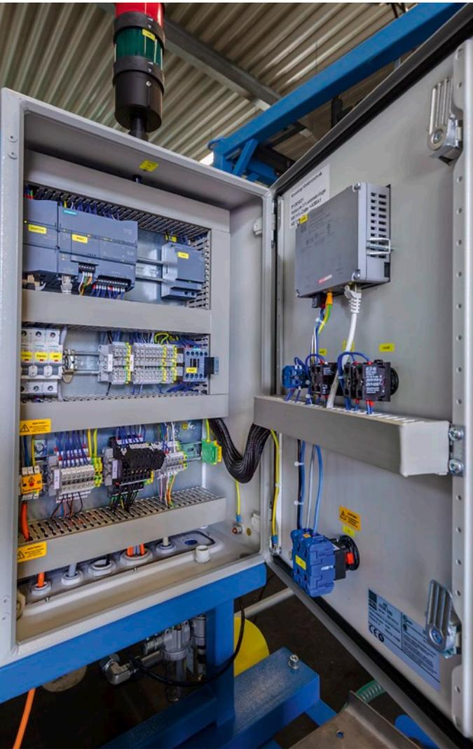
Thanks to Simatic S7-1200 with CPU 1214C, each Infucube works independently
