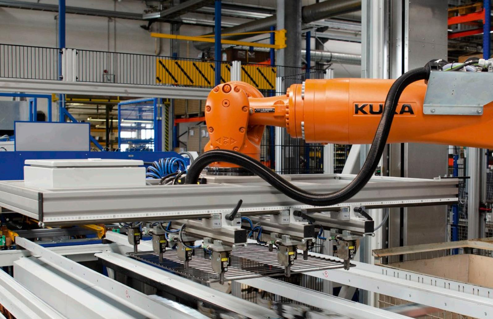
A special gripper lifts the wire frame, rotates it 180° and passes it on to a second gripper
