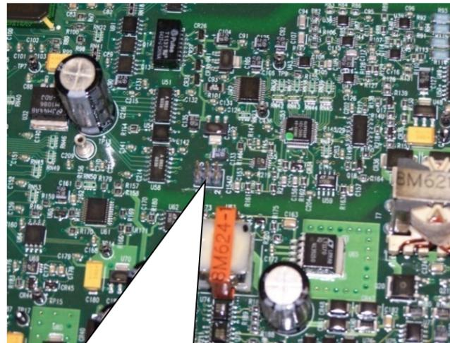
Connect the Lattice upload cable to J-2 on the module. Ensure proper orientation of the cable so pin 6 on the module connects with pin 6 on the cable.
