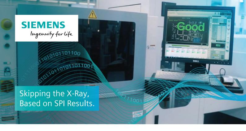
The challenge: X-ray machines are expensive to purchase and operate. In order to reduce costs and not exceed capacity, only a sampling of boards are inserted into the X-ray machine for testing. In the event that the customer (or the customer's customer) requires X-ray tests for the entire batch, the resulting bottleneck will degrade line performance, or lead to investments in additional X-ray machines.
