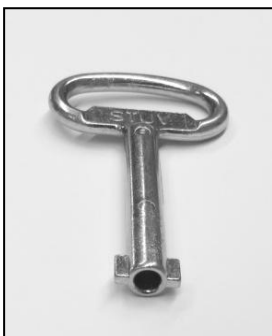
Fig. 25: Double-bit key with a diameter of 5 mm for unlocking and interlocking the withdrawable part / switching-device truck
