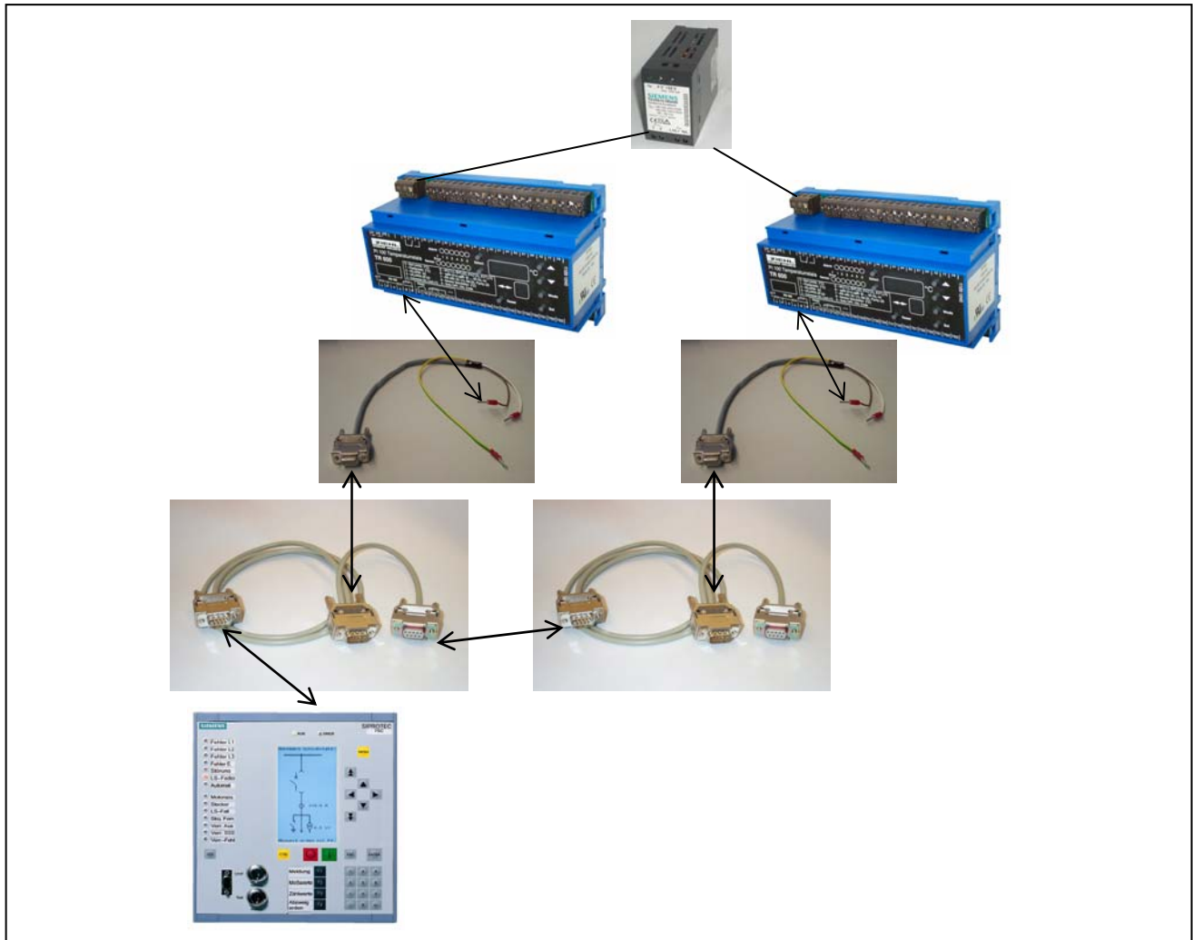
Picture 11: Connection with 2 RTD boxes
