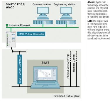
plant's real automation and control systems, for example. Oppelt from Siemens explains: "We can emulate our physical programmable logic controllers and all the communication [systems]. We can connect the original program to a digital twin of the instrumentation with sensors, actuators, motors, and drives, which are all digitally represented."
