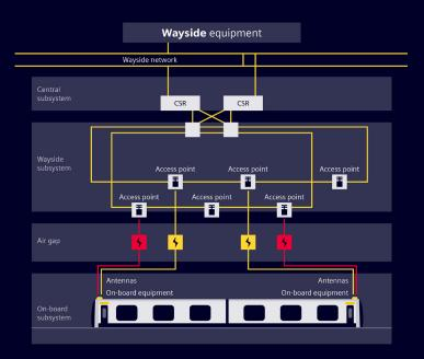
The Airlink radio communication system guarantees a highly reliable seamless and redundant flow of information between the track and a train.
