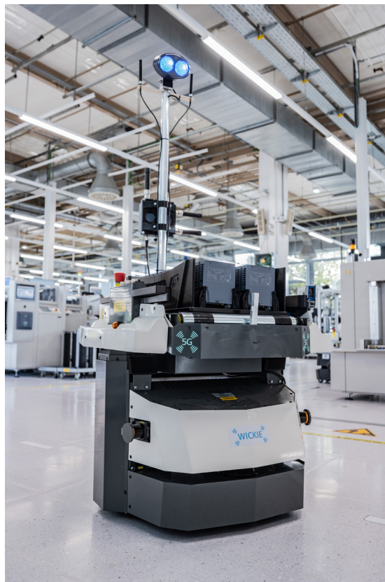
"Wickie", one of MF-K's mobile "cobots" (collaborative robots), delivers semi-finished products – right when they are needed.
