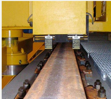
Inductive sensors can measure the offset and steer the crane towards center.
