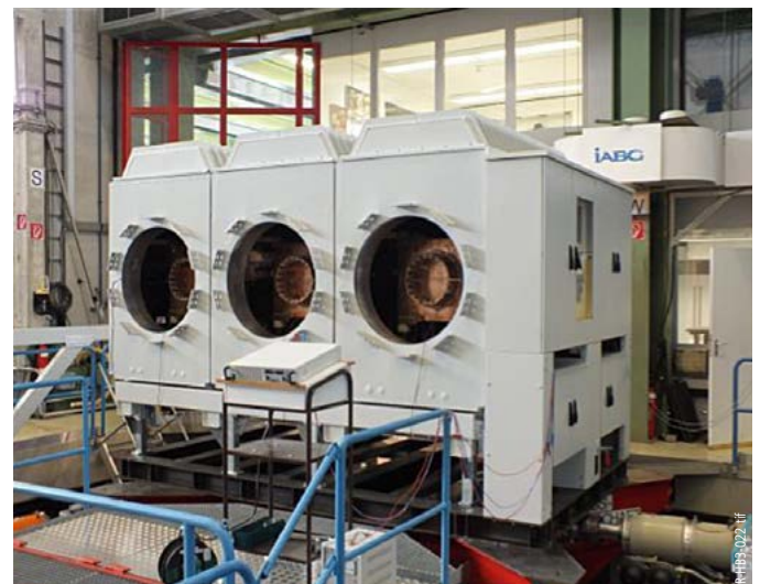
Fig. 52 HB3 switchgear during seismic testing
