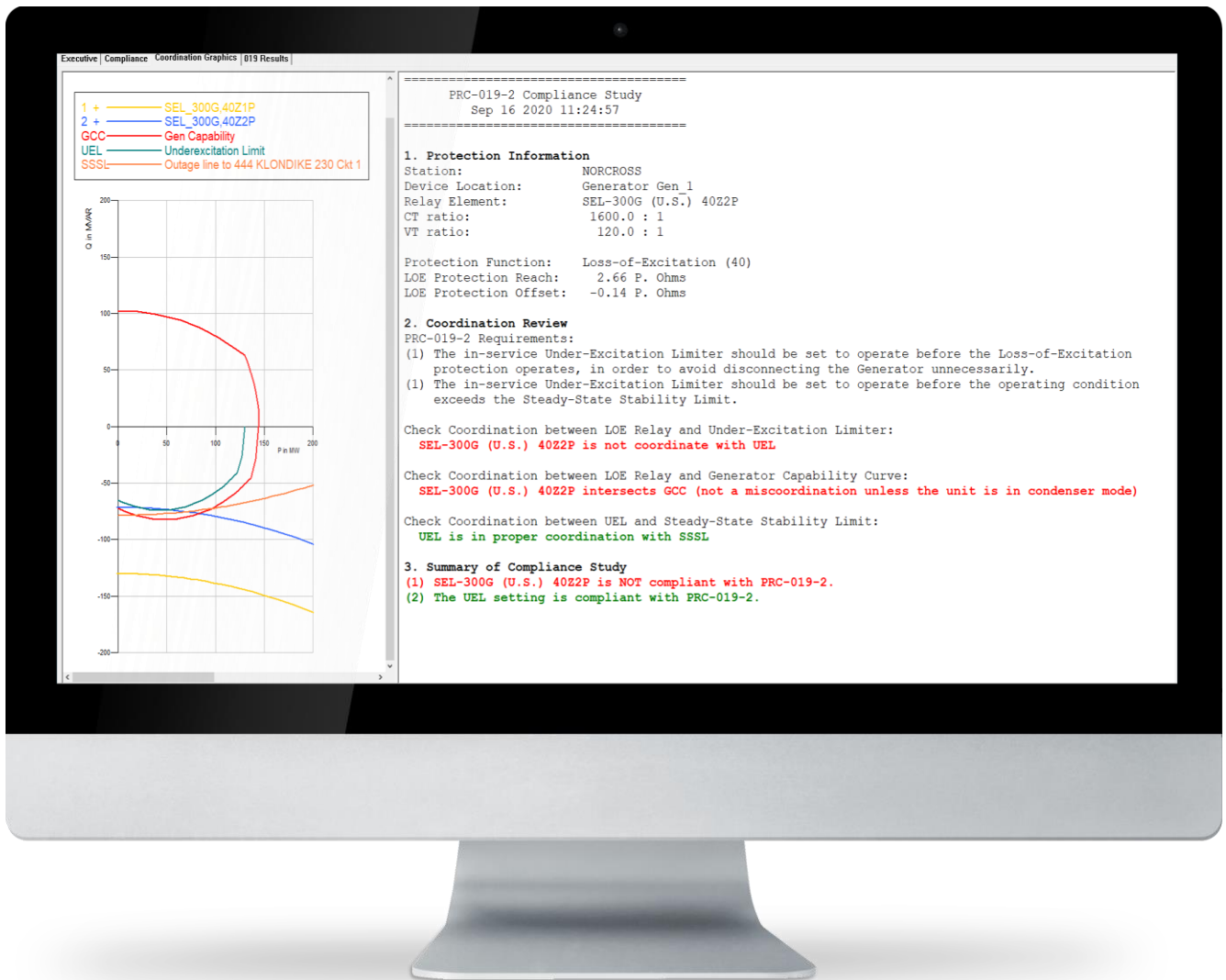
Figure 5: Generator protection coordination with generator controls is automatically evaluated with the Compliance Module.
