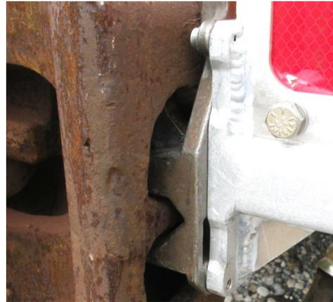
6. Continue to turn the crank handle clockwise until the EOT is snug against the coupler body. Hand tightening the EOT mount is sufficient to secure the EOT in place. **No tools should be used to tighten the EOT mount.**
