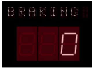
**Figure 5-1 Emergency Braking Display**
