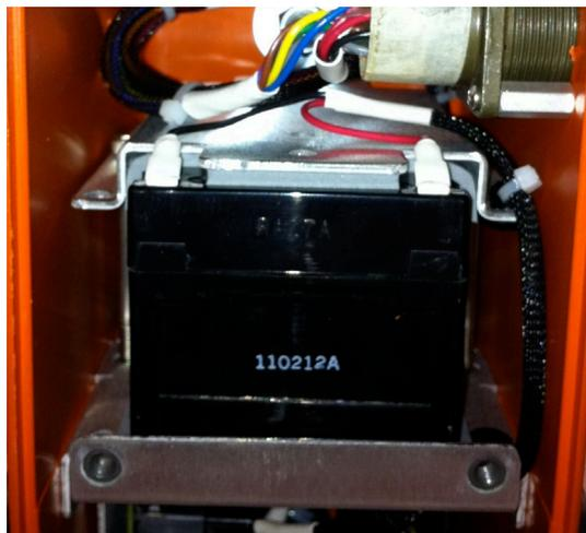
**Figure 9-2 Battery Module Assembly**
