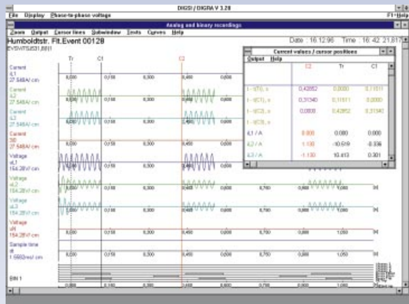
Fig. 5 Fault record of analog and binary traces
