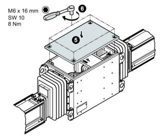
Figure 3-27 Mounting the expansion unit - Figure 10
