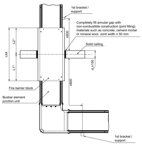
1) In the case of installation off-centre with respect to the solid ceiling, the outer edge of the fire barrier block must be at least 70 mm away from the centre of the ceiling.
