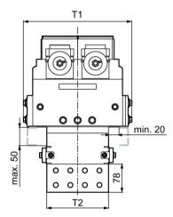
Figure 3-32 Single body system: Busbar connection unit for non-Siemens distribution boards
