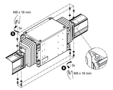
Figure 3-22 Mounting the expansion unit - Figure 5
