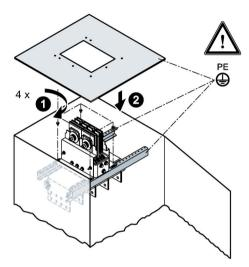
Figure 3-30 Single body system LI-.....-00-FA: Installation in distribution board
