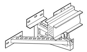
Figure 3-6 Wall fixing for elements of the LI system, mounting position "flat"
