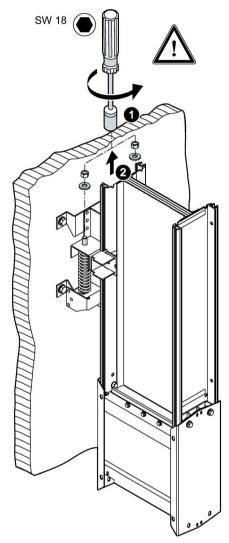
Figure 3-10 Mounting the busbar trunking system on a bracket for vertical installation - removing the adjustment screws
