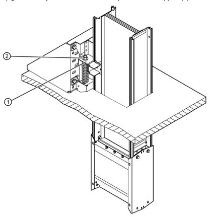
Figure 5-1 Brackets for vertical installation
