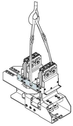
Figure 3-29 LI-.....-00-FA1.., LI-....-00-FA2..: Transporting the busbar connection unit for non-Siemens distribution boards
