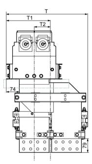
Figure 3-33 Double body system: Busbar connection unit for non-Siemens distribution boards
