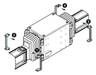
Figure 3-20 Mounting the expansion unit - Figure 3
