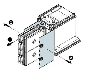
Figure 3-46 Replacing insulating plates - Figure 2
