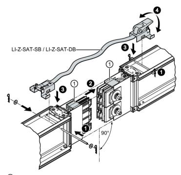
① Spacers are not removed until the insulating plates have been pushed inside one another by about 2 cm and before the busbar conductors have been moved to their final position.
