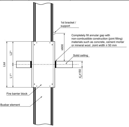
In the case of installation off-centre with respect to the solid ceiling, the outer edge of the fire barrier block must be at least 70 mm away from the centre of the ceiling.
