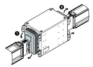
Figure 3-18 Mounting the expansion unit - Figure 1
