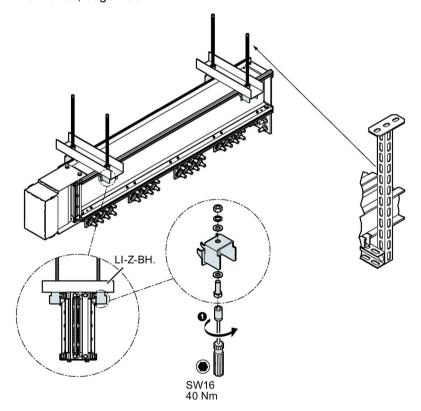
Figure 3-17 Ceiling fixing
