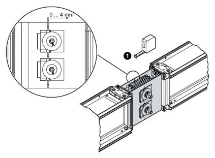
Check the clearance between both trunking units. Their clearance on the earthing guide plates may be within a tolerance range of 0 to max. 4 mm. Then, the hook and bolt connection is adjusted correctly.
