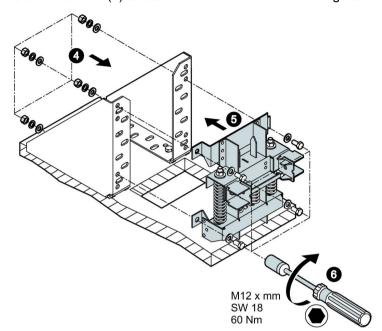
2. Use the screws (4) to attach the additional vertical flange to a module.
