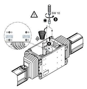
Figure 3-26 Mounting the expansion unit - Figure 9
