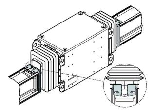
Figure 3-21 Mounting the expansion unit - Figure 4
