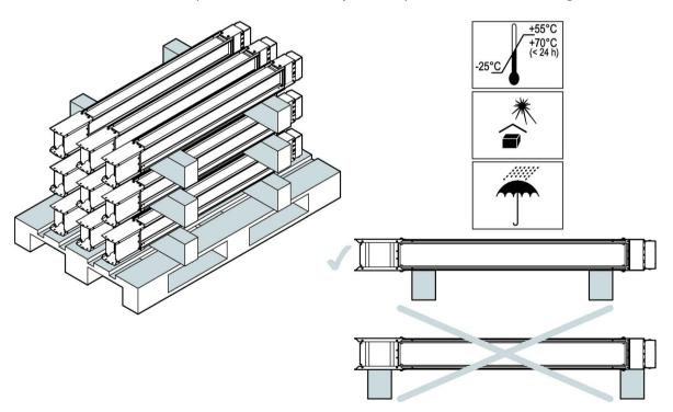
Figure 2-1 Storing straight trunking units
