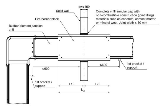
1) In the case of installation off-centre with respect to the solid wall, the outer edge of the fire barrier block must be at least 70 mm away from the wall's centre.
