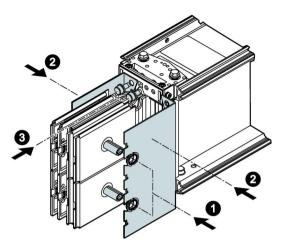
Figure 3-49 Replacing insulating plates - Figure 5
