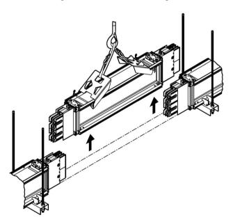
Figure 5-2 Dismantling the trunking unit
