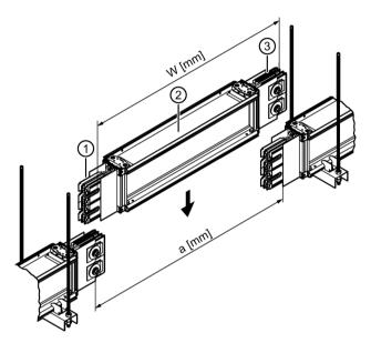
Figure 3-1 Assembly: straight trunking unit as last element in the busbar run
