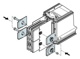
Figure 3-50 Replacing insulating plates - Figure 6
