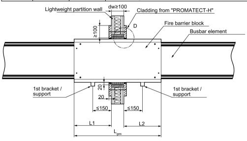
Figure 3-37 Partitioning of the LI busbar system in a lightweight partition wall
