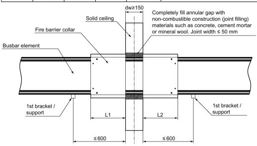
Figure 3-42 Partitioning of the LI busbar system in a solid wall - Figure 4
