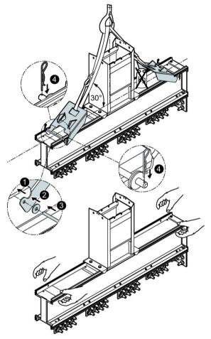
Figure 3-34 Transformer connection units
