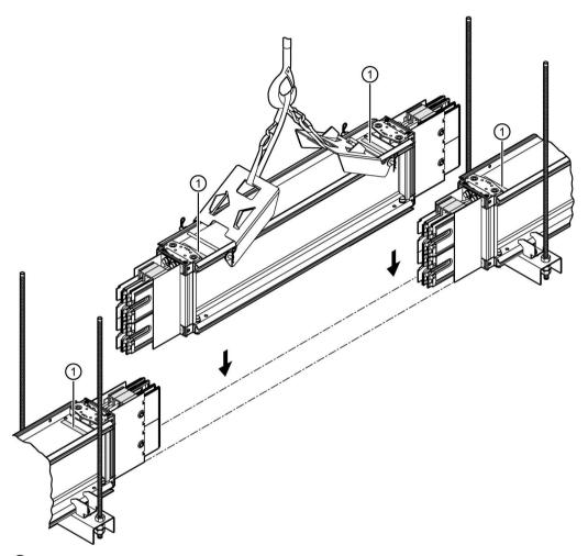
① Attention: check conformity of the conductor configurations.
