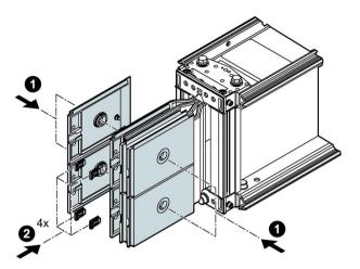
Figure 3-48 Replacing insulating plates - Figure 4
