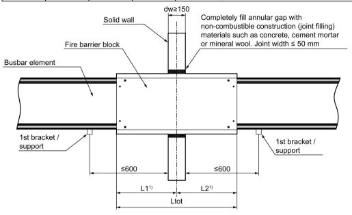
1) In the case of installation off-centre with respect to the solid wall, the outer edge of the fire barrier block must be at least 70 mm away from the wall's centre.
