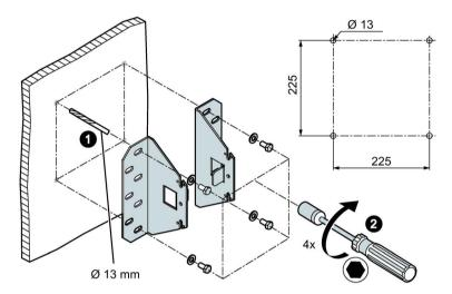
Figure 3-15 Mounting the fixing brackets with fixed point for vertical installation - Figure 1
