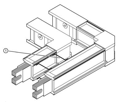
① Connecting with spacers (final mounting state)
