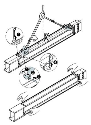
Figure 2-3 Single body system: Suspension from slings with crane fixture / transport for horizontal busbar runs
