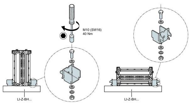
Figure 3-4 Fixed-point brackets attached to solid building structure: horizontal edgewise on left; horizontal flat on right
