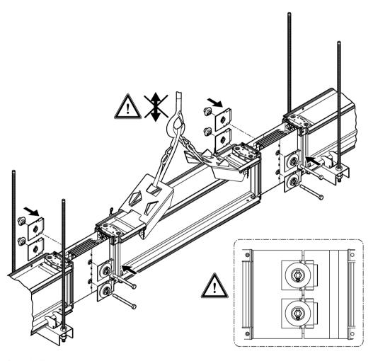
Step 8: Tightening connecting bolts, mounting side and cover plates
