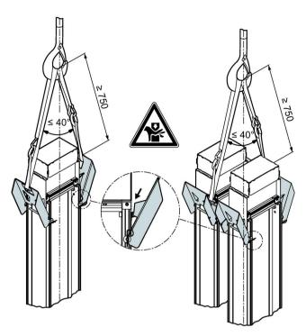
Figure 2-5 Suspension from slings for vertical busbar runs
