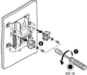
Figure 3-8 Mounting the bracket for vertical installation on the wall - Figure 2
