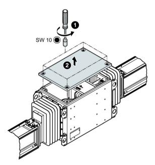
Figure 3-25 Mounting the expansion unit - Figure 8
