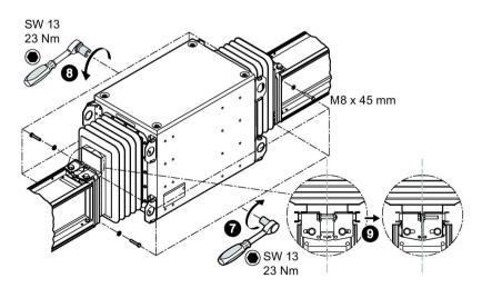
Figure 3-23 Mounting the expansion unit - Figure 6
