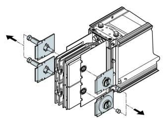
Figure 3-45 Replacing insulating plates - Figure 1
