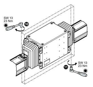
Figure 3-24 Mounting the expansion unit - Figure 7
