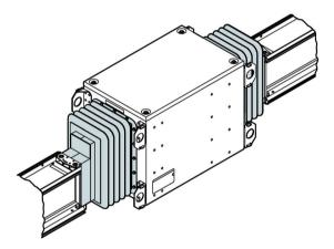
Figure 3-19 Mounting the expansion unit - Figure 2
