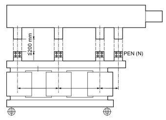
Figure 3-35 Positioning the transformer connection unit
