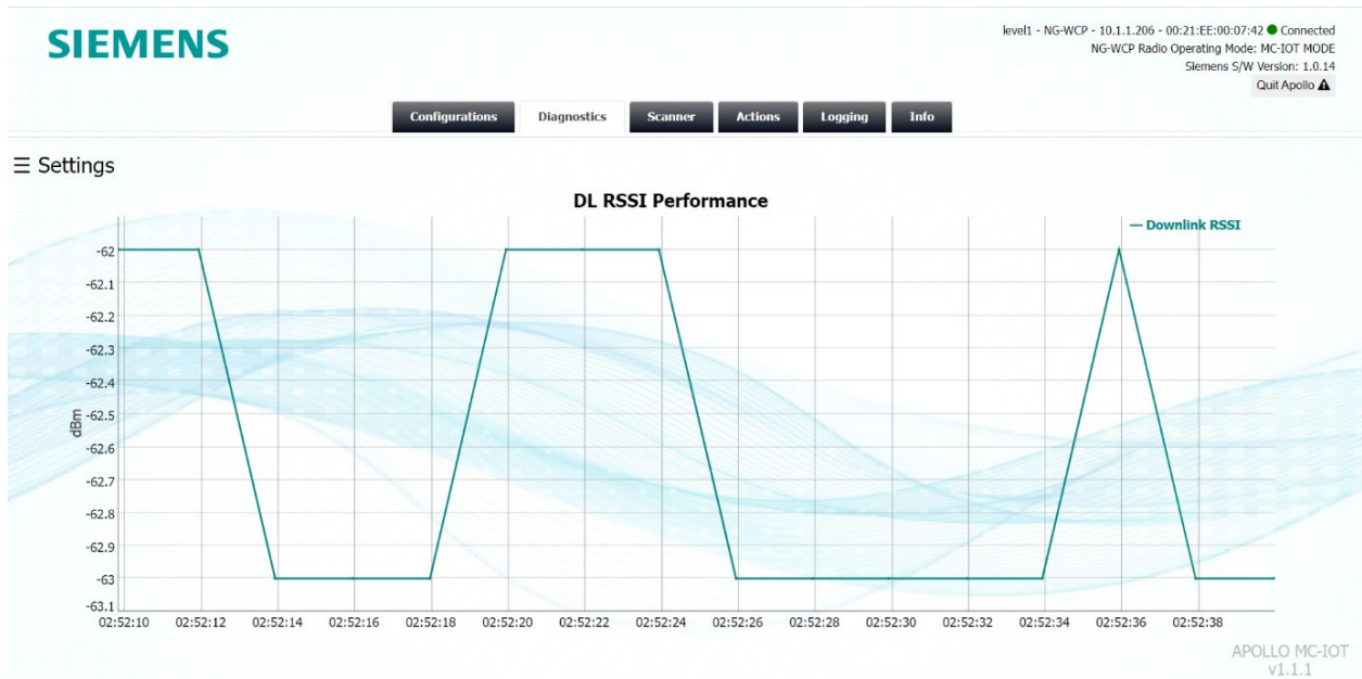
Figure 7-12 Diagnostics Screen – One Graph Plotting (in MC-IoT Mode only)
