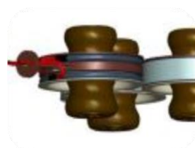
2 x Rogowski Coils for Current Measurement (redundant)
