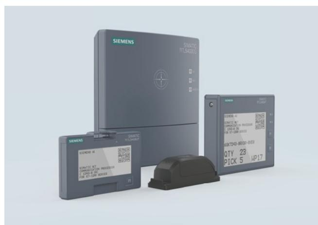
Locating systems consist of different transponders (front left: with e-paper display for dynamic display of information, front right: for production resources) as well as a network of gateways (back) that then provide information to the locating server.
