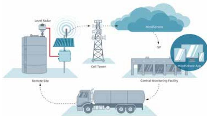
*Siemens remote tank monitoring puts tank data at your fingertips with secure wireless communications, an extensive instrumentation portfolio and Insights Hub.*
