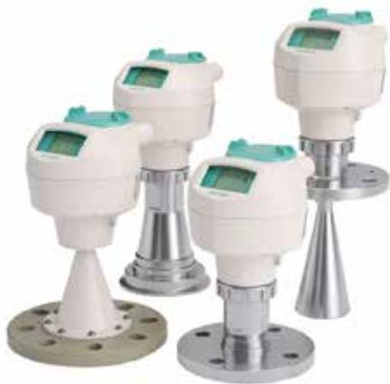
*SITRANS LR250 is a 2-wire, 25 GHz pulse radar level transmitter for continuous monitoring of liquids and slurries in storage and process vessels including high temperature and pressure, to a range of 20 m (66 ft).*
