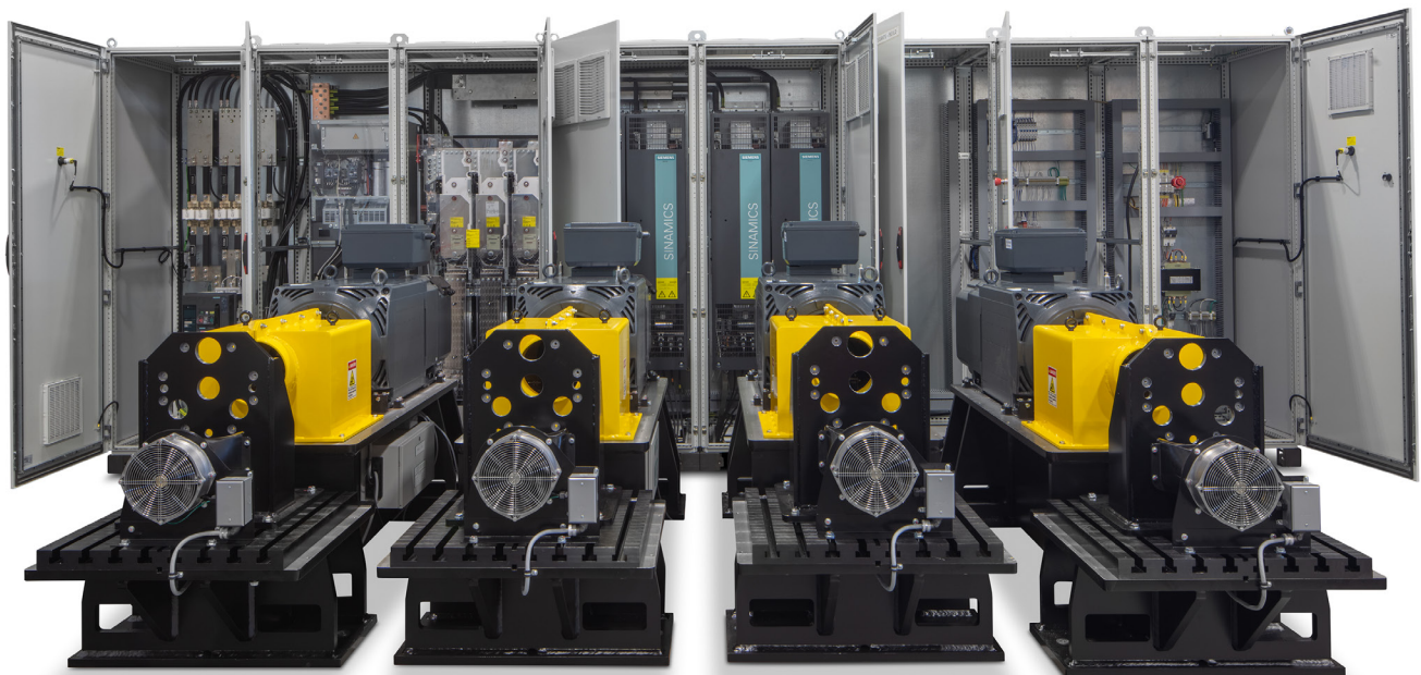
ACS used Siemens SINAMICS S120 drives and asynchronous SIMOTICS M-1PH8 induction motors
