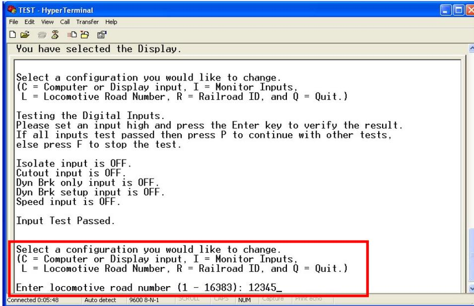
3. Press the **Enter** key on PC keyboard to save the locomotive road number to the configuration file and return to the configuration edit selection prompt.
