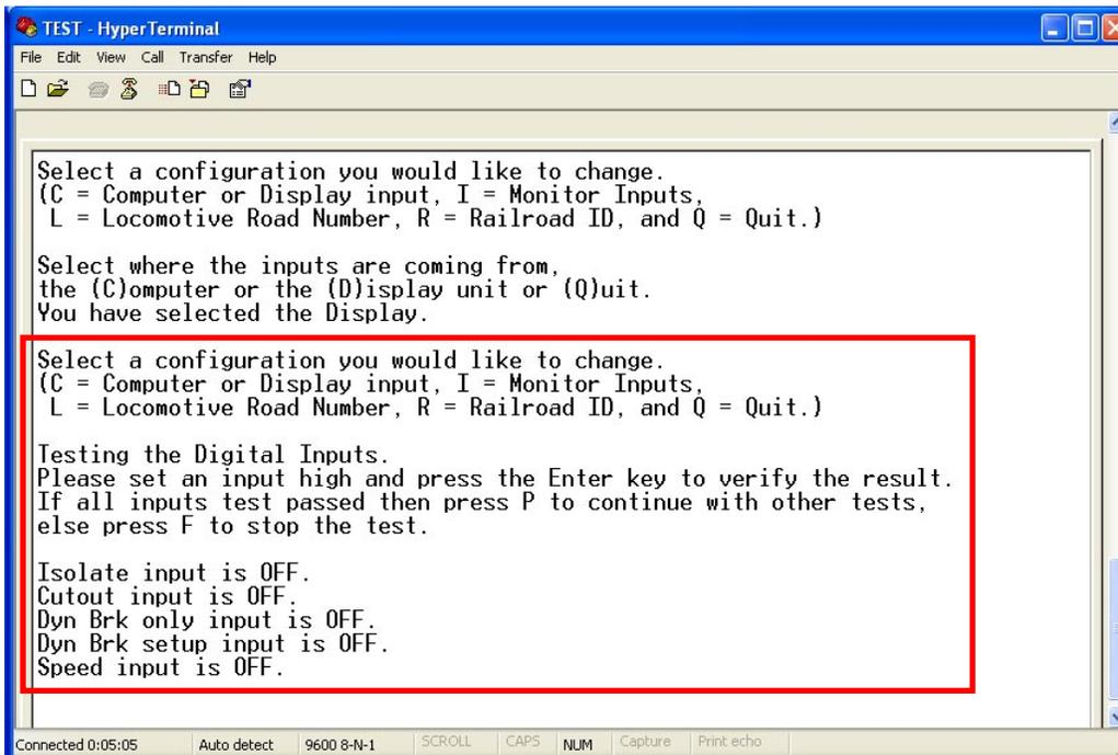
2. To view current input status, press the **Enter** key on the PC keyboard. The current condition of each input is displayed at the bottom of the screen.
