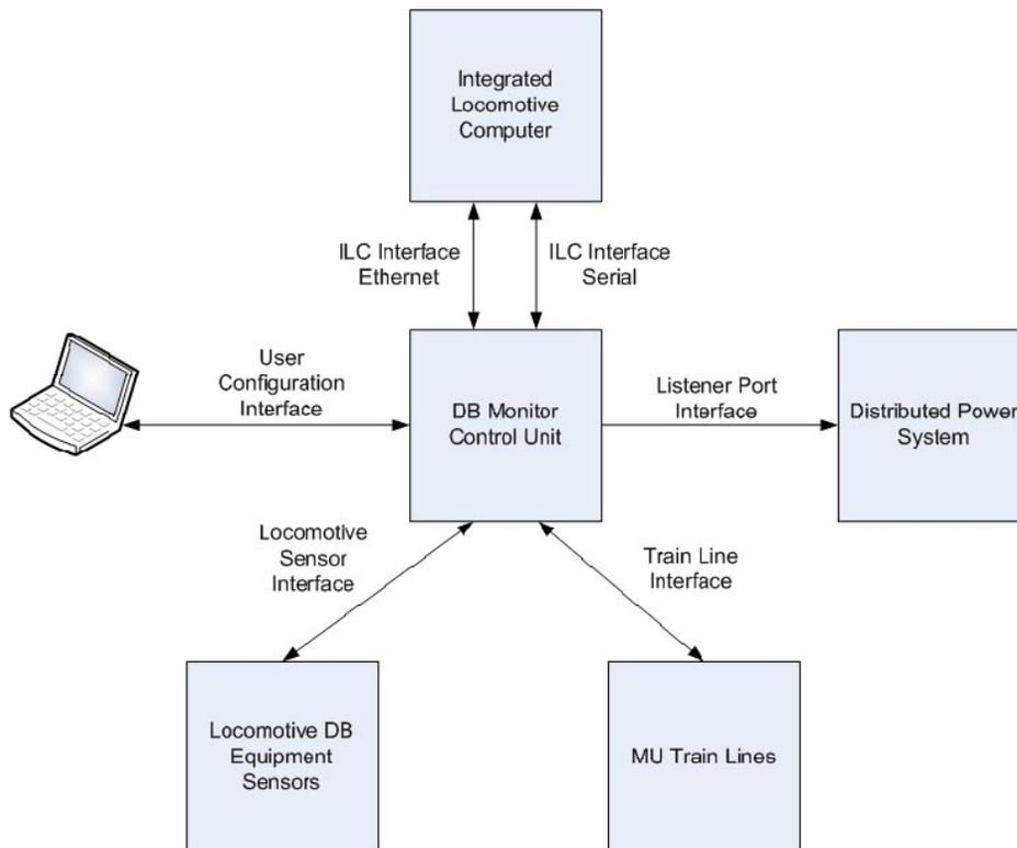
Figure 2. Dynamic Braking Monitor System Context
