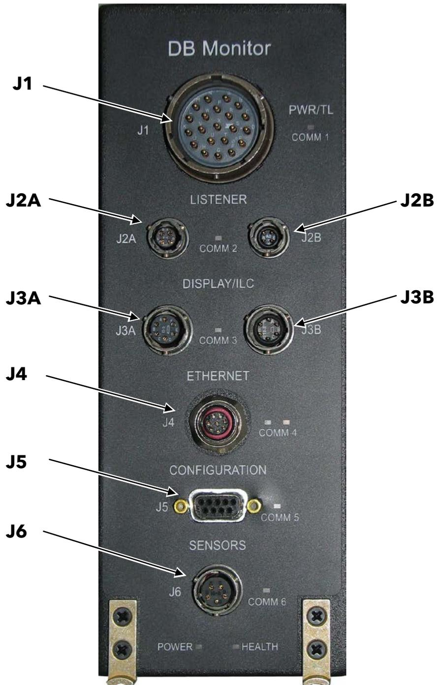
Figure 3. DBM Connector Locations
