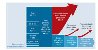
Energy Flows in the <u>Global</u> Electricity System, ~65% of total energy input is lost
