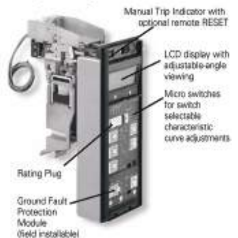
Sample Configuration of an ETU745
