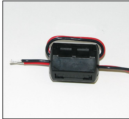
Figure A-3 EMI Filter Installed
