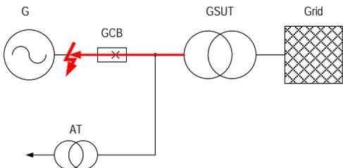
Fig 2. System-source short-circuit
