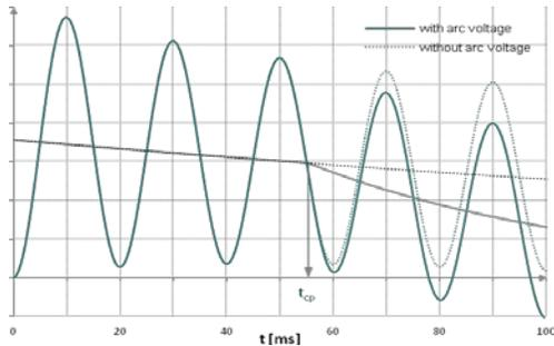
Fig 6. Principle effect of arc voltage at contact parting
