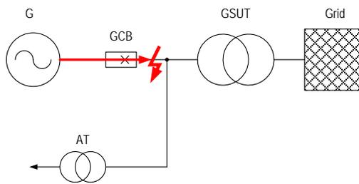
Fig 4. System-source short-circuit
