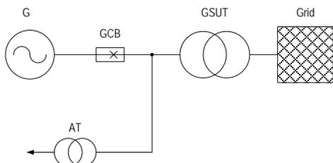
Fig 1. Typical layout of a generator circuit
