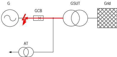
Fig 2. System-source short-circuit
