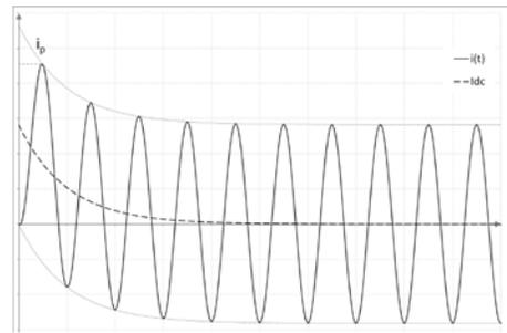
Fig 3. Typical current curve of a system-source fault
