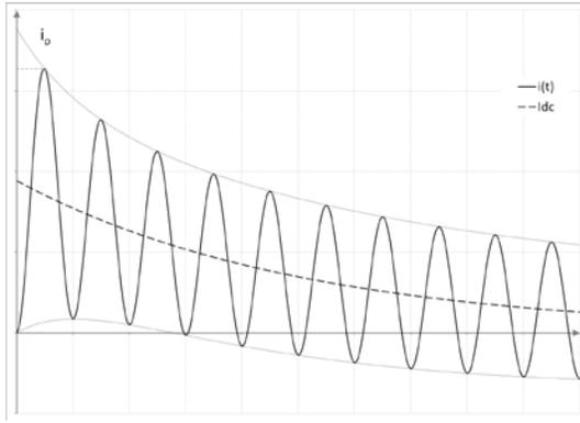
Fig 5. Typical current curve of a generator-source fault
