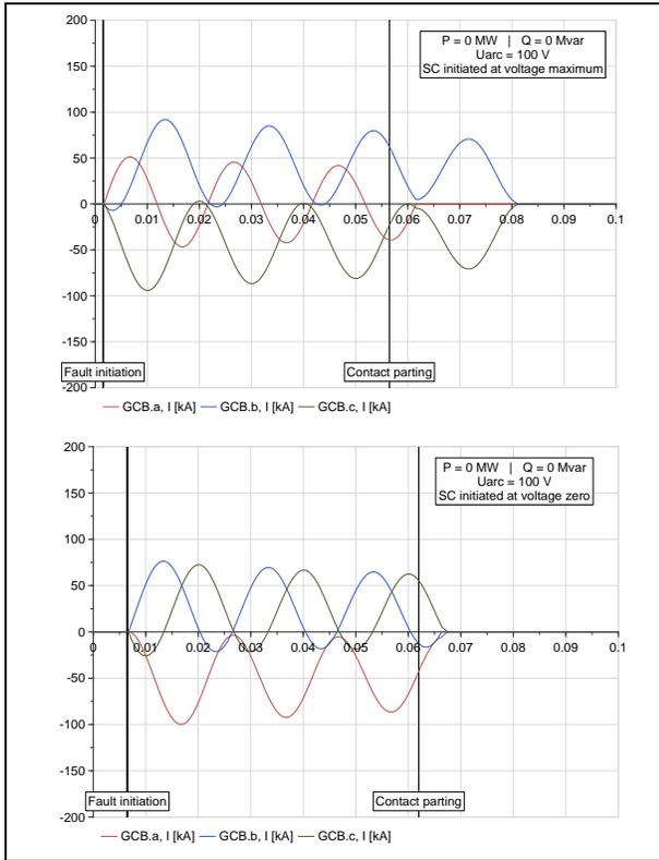
A 1. Generator-source fault current – generator at no load
