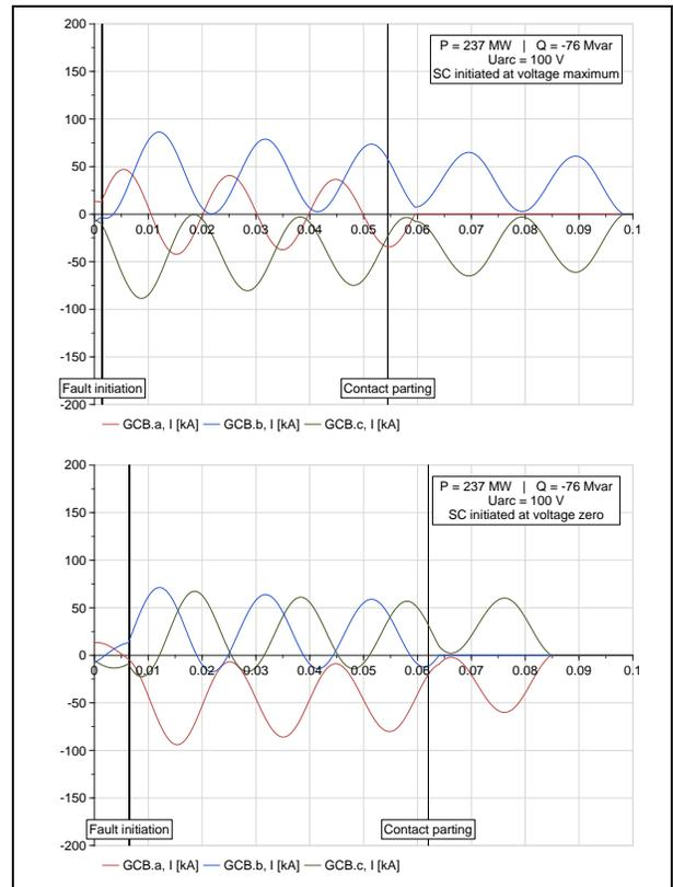
A 3. Generator-source fault current – generator in leading mode
