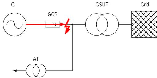
Fig 4. System-source short-circuit
