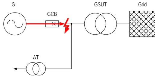
Fig 4. System-source short-circuit
