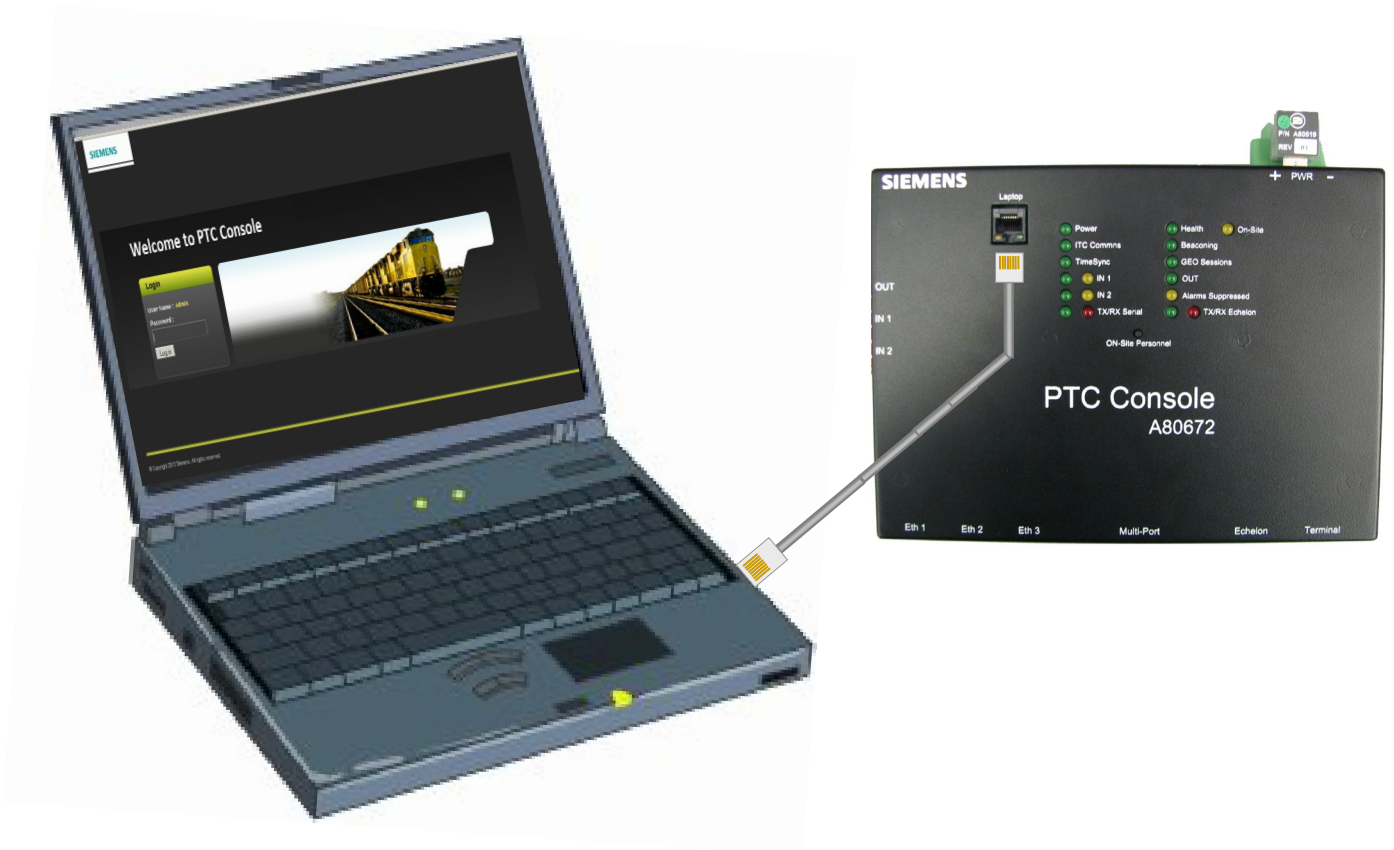
Figure 3-8 Laptop Connection to the PTC Console
