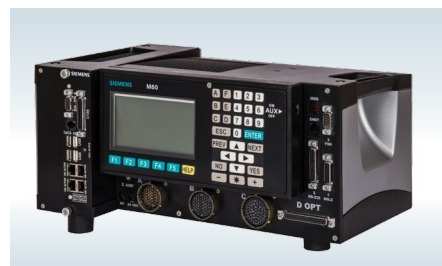
Siemens M60 ATC controller running SEPAC local controller software
