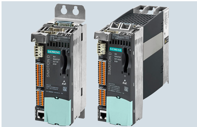
Left: SIMOTION D410-2 Control Unit attached to mounting plate
