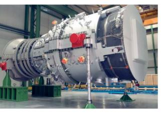
The SGT5-8000H – the largest and most powerful gas turbine in the world. After the test phase in Irsching, near Ingolstadt in Bavaria, the system will be expanded into a high-efficiency combined cycle power plant with an output of approximately 530 megawatts and efficiency of over 60 percent.
