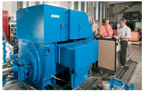
further development of this energysaving technology and uses wires made of superconducting material for the windings of electric machines, among other applications. This improves the efficiency of motors and generators.
