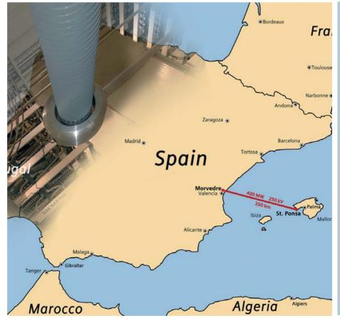
several hydroelectric power plants will be transported over this 1,400-kilometer (870-mile) direct-current link. Hydroelectric power generation is economical, environmentally friendly, and does not emit any carbon dioxide. This HVDC link will help to prevent the emission of over 30 megatons of climate-damaging carbon dioxide a year that would have been produced with conventional, local power generation.
