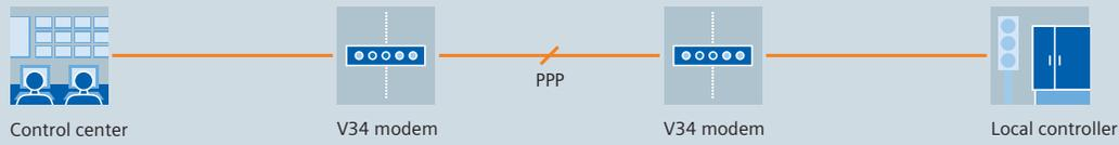
Dedicated line operation via V.34 interface and PPP/TCP/IP protocol: the ideal solution for existing cabling in all cases where relatively low data transmission capacity is adequate
