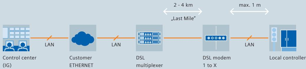
Dedicated line operation via Ethernet/DSL link: several times faster than a V.34 link and no need for modem cabinet
