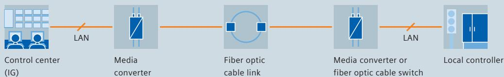
Dedicated line operation via Ethernet/fiber optic cable link: speeds of up to 1Gbit/s and zero susceptibility to electromagnetic interference
