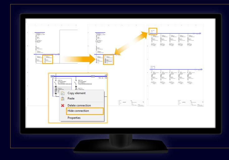
Another option is to hide the connections from distributors by marking the connection in the network plan and selecting Hide the connection in the context menu. A cross reference is being created and by clicking on the **symbol**  $\bigtriangleup$  you can jump to the connected part. This is another way to design a well-organized network plan. The connection can be reestablished immediately by right-mouse-click.
