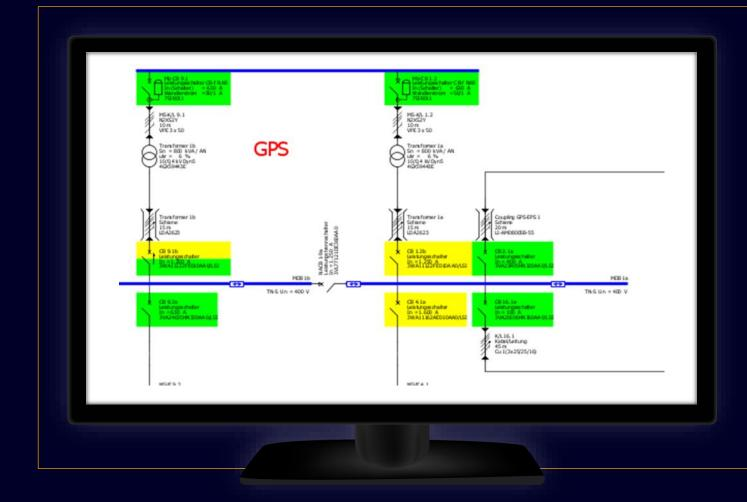
In addition, each switching device is colourmarked in the entire network diagram as follows, when selectivity evaluation was enabled:
