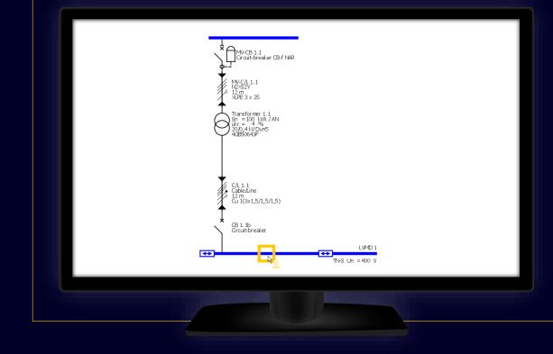
Parallel infeed using several power sources can be mapped by placing more infeed components at an insert point on the busbar and specifying them in the dialog displayed afterwards.
