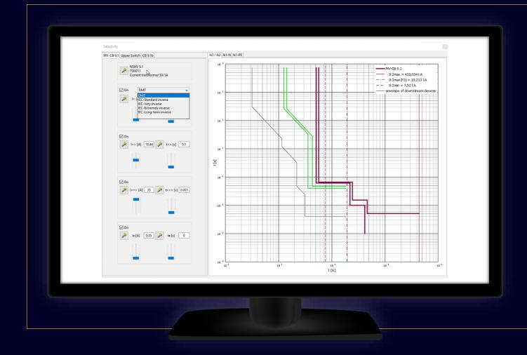
For medium-voltage circuit breakers you can select either DMT (Definite Minimum Time) or IDMT (Inverse Definite Minimum Time) in the selectivity window
