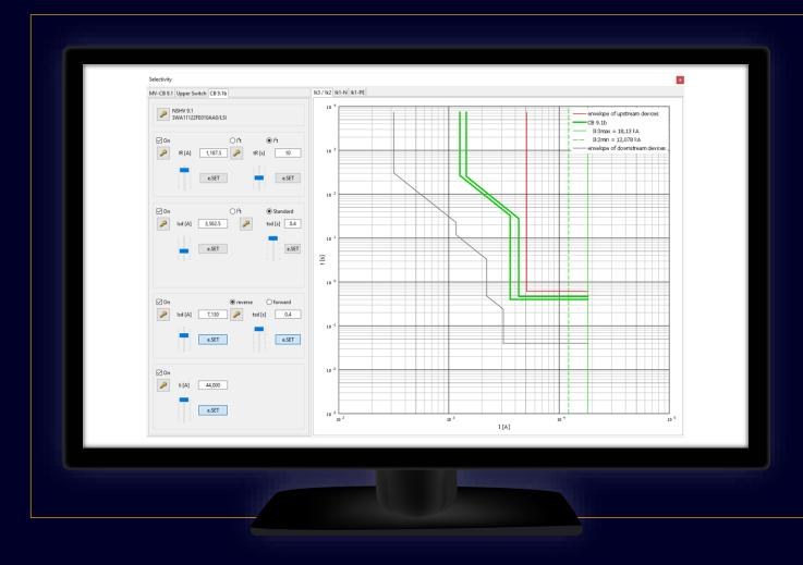
For type 3WA open circuit breakers, in addition to the known settings for LSIG, a directional short circuit protection (dst) can also be set in the "Selectivity" window.
