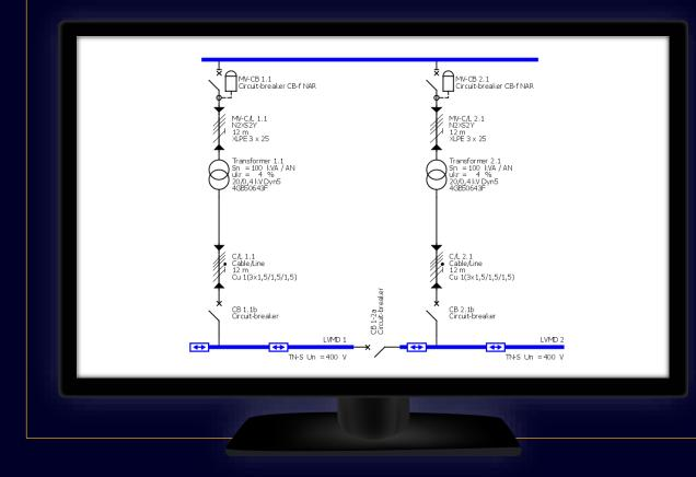
Now you can add distribution boards and load circuits to the new busbar for the new feed-in system linked by the coupling in the usual way.
