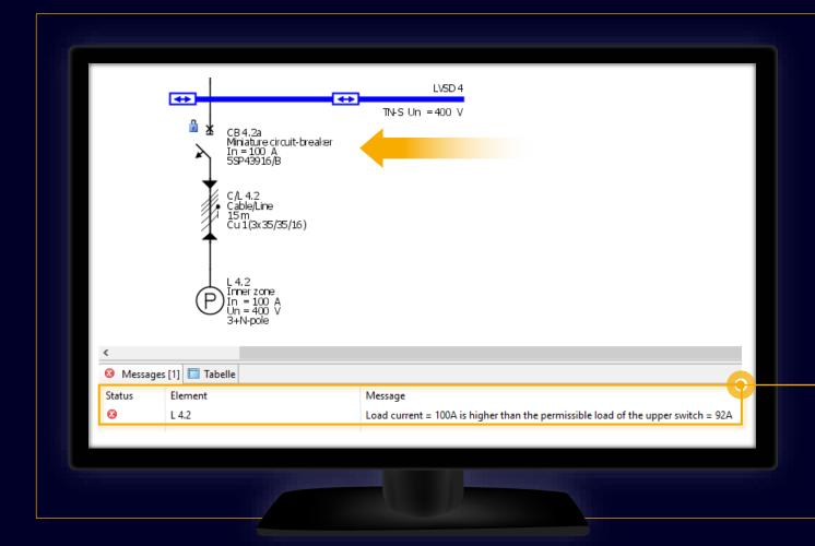
If errors should occur during the dimensioning process, e.g. owing to default devices which do not meet the requirements for the defined operating modes, info and error messages will be displayed below the network diagram.
