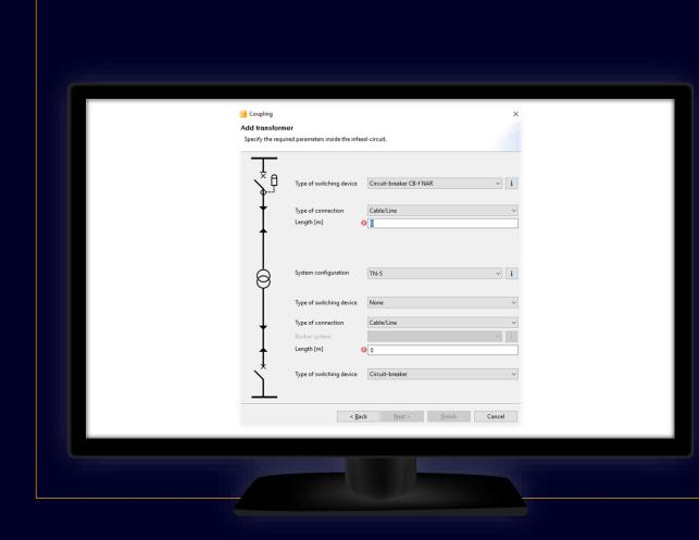
Now you must define the data required for the selected type of second infeed, in this case it is a transformer without medium voltage.
