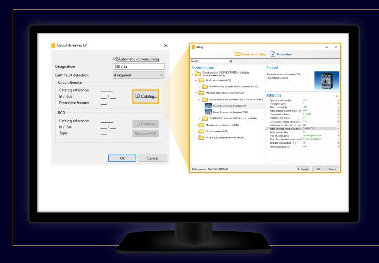
**Devices** can be manually specified again, e.g. after their "**Properties**" were called up from the product catalogue integrated into the software.
