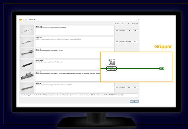
Having selected the busbar trunking system and defined its length, you can graphically edit it on the network diagram, e.g. by dragging the gripper with the mouse, thus elongating the busbar in the diagram.
