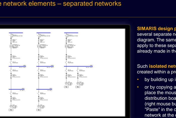
SIMARIS design professional allows to create several separate networks on the network diagram. The same medium-voltage specifications apply to these separate networks that were already made in the project definition.
