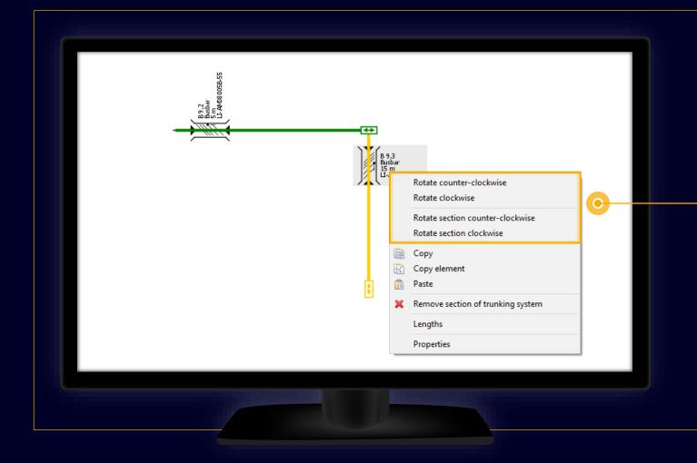
You can also adjust the graphical layout of busbars by calling up the corresponding functions for rotating the marked section, or rotating the entire busbar layout, from the context menu with a right mouse click.
