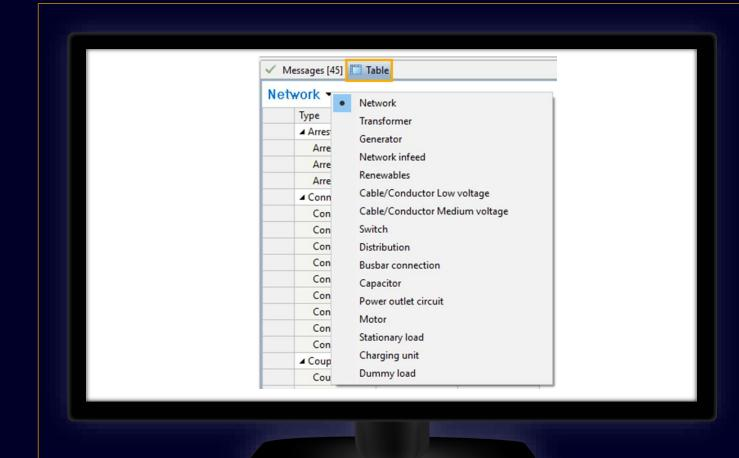
In order not to lose the overview in an extensive network map, SIMARIS design offers a comfortable **table view**, which you can call up by clicking the button below the network.
