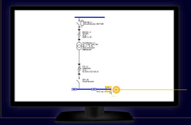
In order to add a general coupling for normal power supply to the network diagram, please note that the cursor must placed at the **outer end** of the busbar node of the feed-in circuit.
