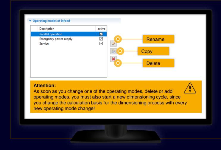
More operating modes are defined by duplicating the existing operating mode. Afterwards the switch positions are defined according to the new operating mode requirements.
