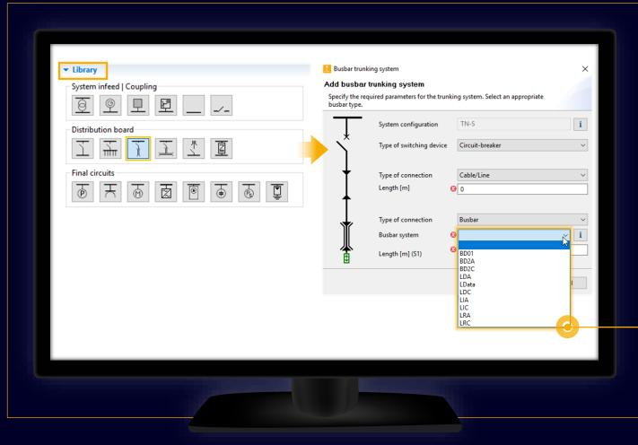
SIMARIS design also helps you integrate busbar systems for power transmission and distribution into your planning concept and displays them on the network diagram.
