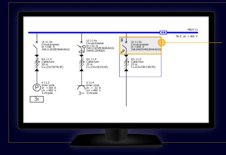
After you have dimensioned the network you created, you can display the characteristic device curves.
