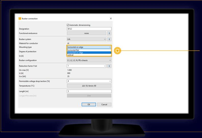
More busbar properties, such as degree of protection and mounting type, can be modified at any time.
