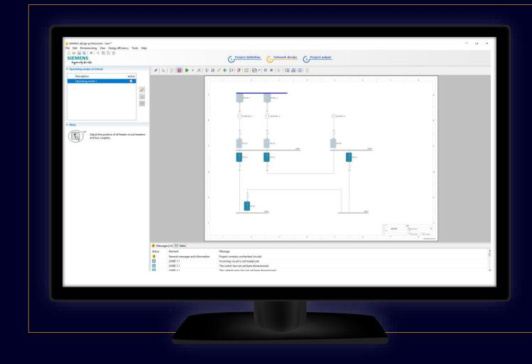
First a view opens in which all switches of sources and distributors can be switched. The switches of the sources are all open, the switches of the distributors are all closed. By clicking on the switch it can be opened or closed.
