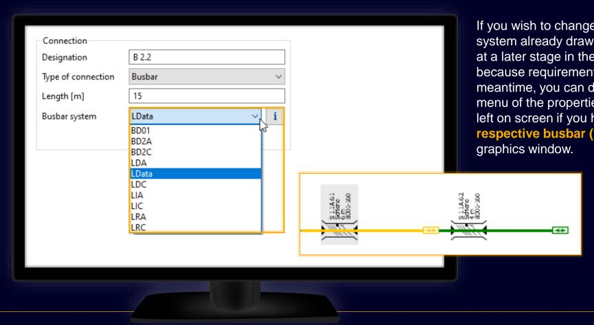
If you wish to change the type of a busbar system already drawn on the network diagram at a later stage in the planning process, because requirements have changed in the meantime, you can do so in the drop-down menu of the properties displayed at the bottom left on screen if you have marked the **respective busbar (yellow line)** in the graphics window.
