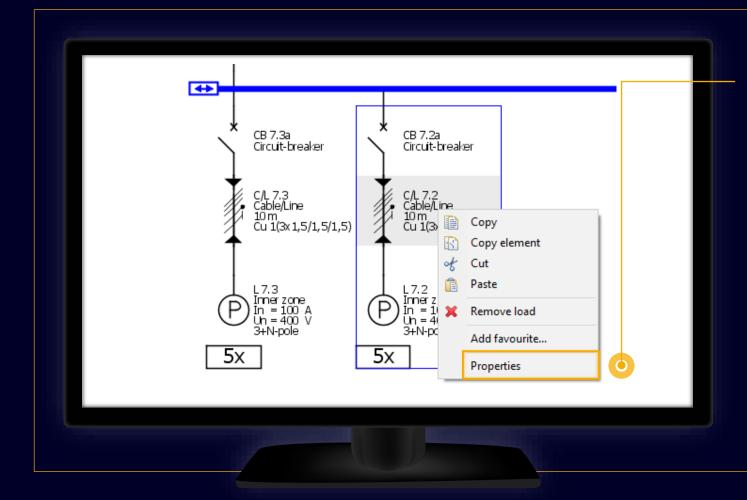
Another possibility is opening the "**Properties**" window by marking the element on the network diagram and selecting "Properties" from the context menu (right mouse button).
