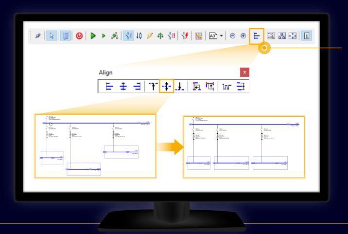
There are more automatic functions for aligning elements on the network diagram which can also be called up from the tool bar.
