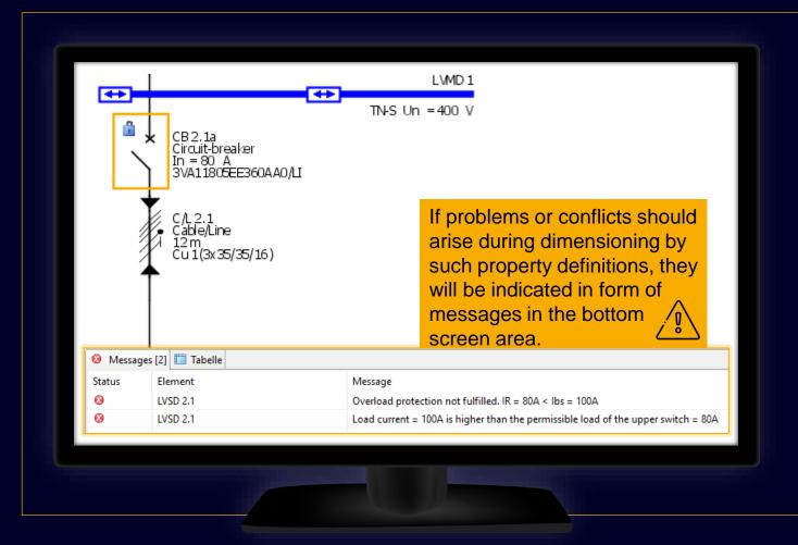
A specific selection in the product catalogue dismisses the automatic device selection, and the manually specified switching device will not be modified by the next dimensioning of the network.
