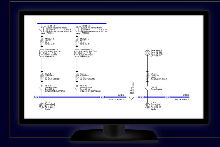
The possibility to dimension identical power sources connected in parallel and calculating the impact of this configuration on the shortcircuit currents or load currents in the network, is extended by another option in SIMARIS design professional:
