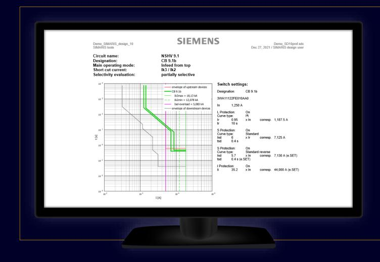
In addition, users of the **professional** version are provided with a selectivity evaluation of every device and the selectivity limits for the device are shown on the graphics.
