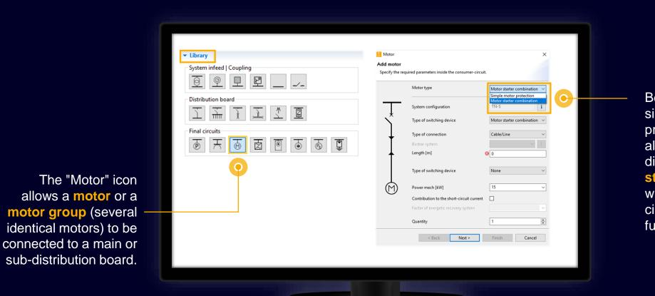
Besides mapping simple standard motor protection, you can also select and dimension motor starter combinations which are protected by circuit-breakers or fuses.
