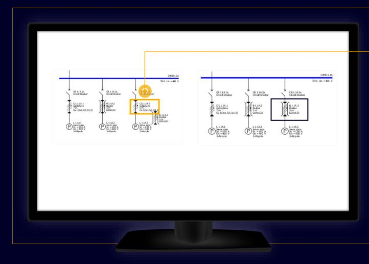
...Then left-click to place it in the desired circuit as a substitute for the previously displayed item. Suitable elements on the network diagram that can be replaced are marked by a yellow frame upon mouseover.
