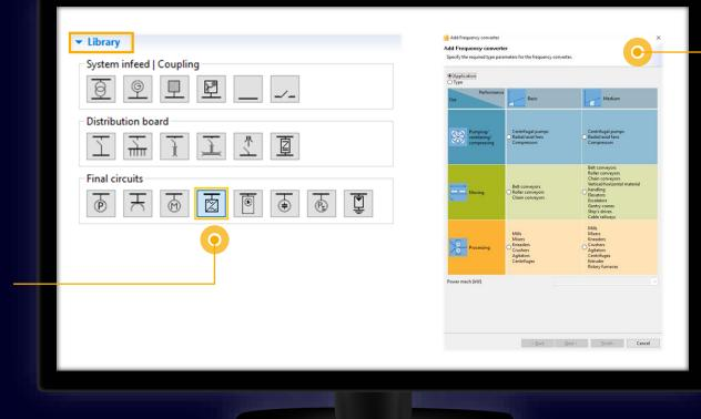
The type of **frequency converter** will be determined automatically by selection of classification, application and power.
