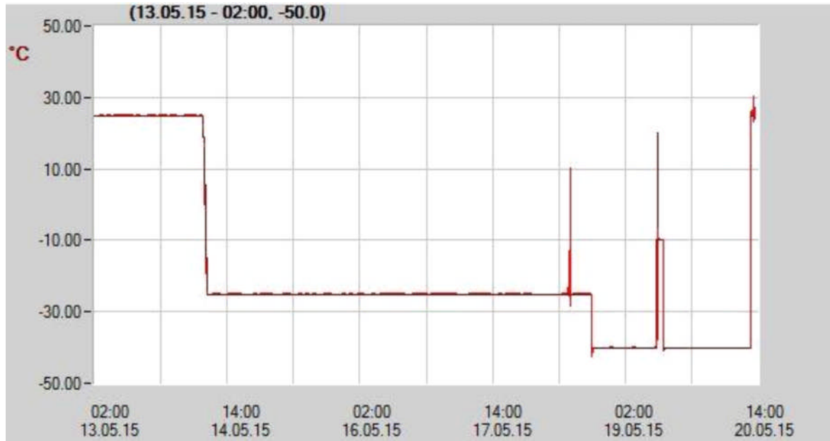
Diagram 2: Stress sequence of the climate tests according to clause 2.1.3 and clause 2.1.4 (test Ab: Cold)
