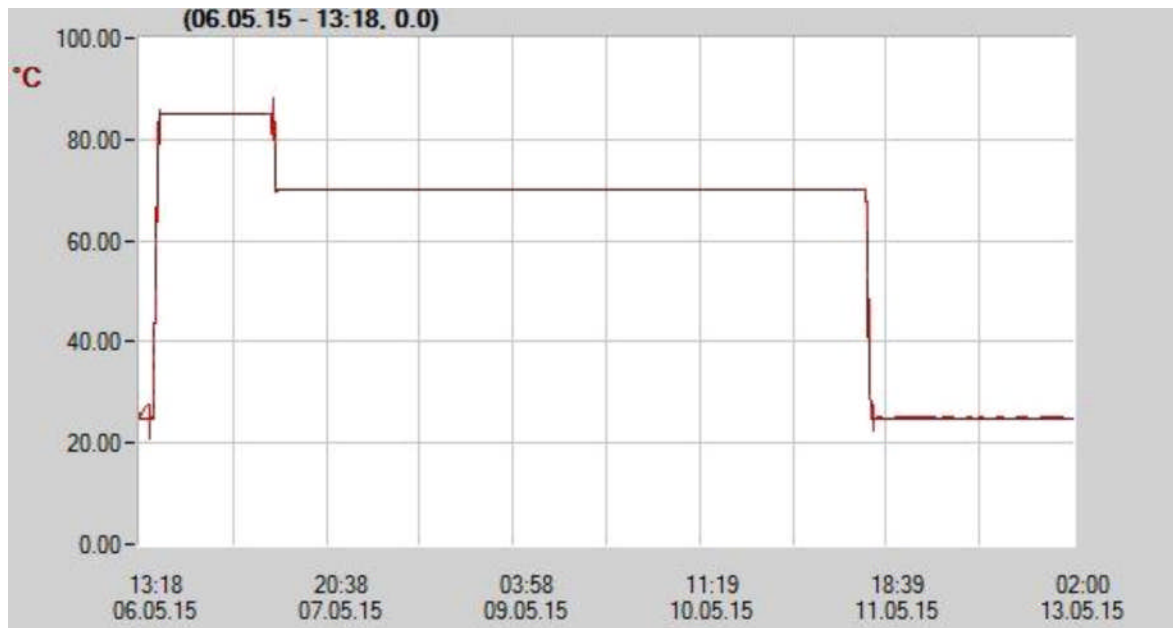
Diagram 1: Stress sequence of the climate tests according to clause 2.1.1 and clause 2.1.2 (test Bb: Dry heat)
