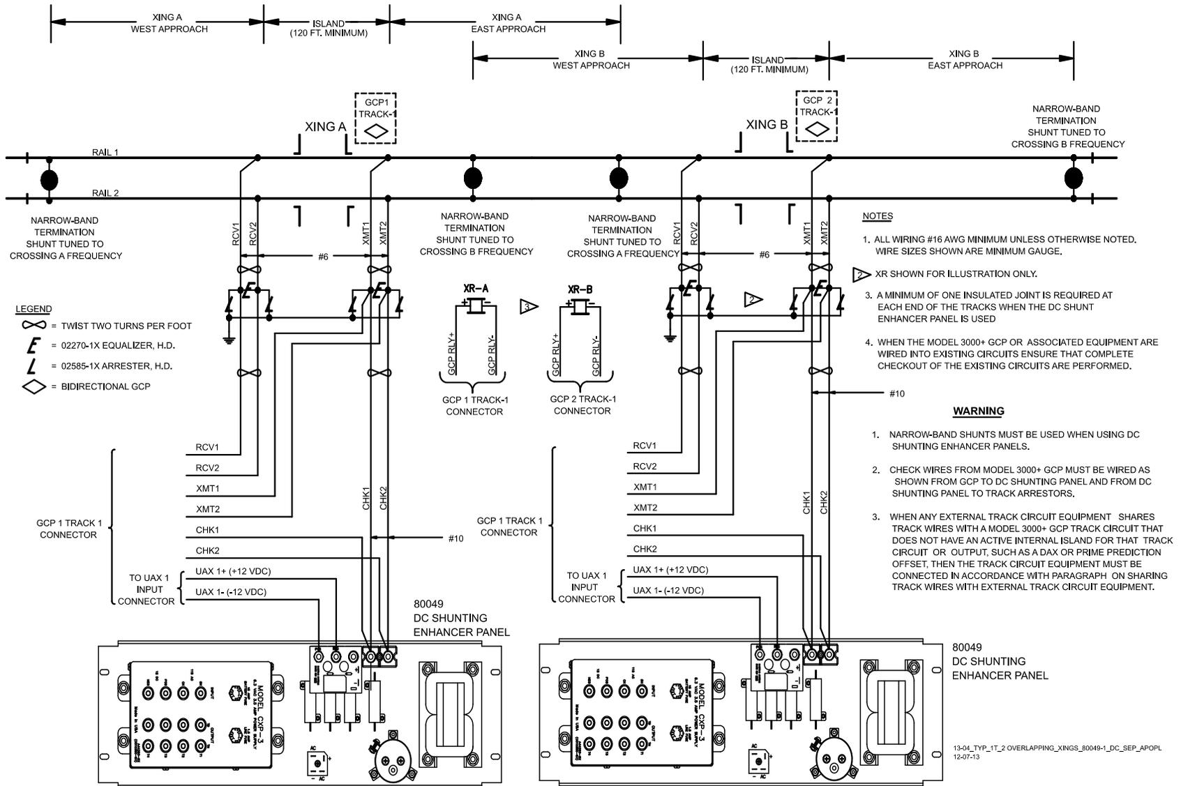
Figure 6-8 DC Shunting Enhancer Panels for Overlapping Crossings
