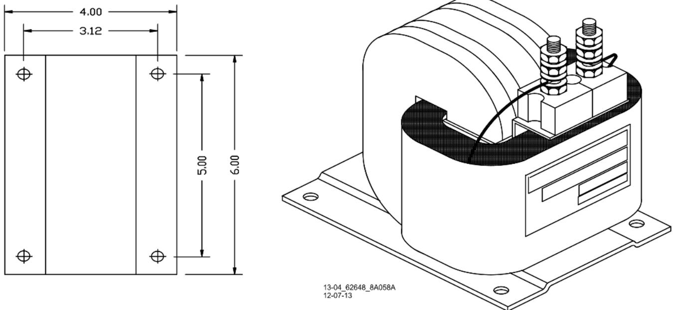
Figure 6-21 Battery Choke with Mounting Dimensions, 62648/8A065A
