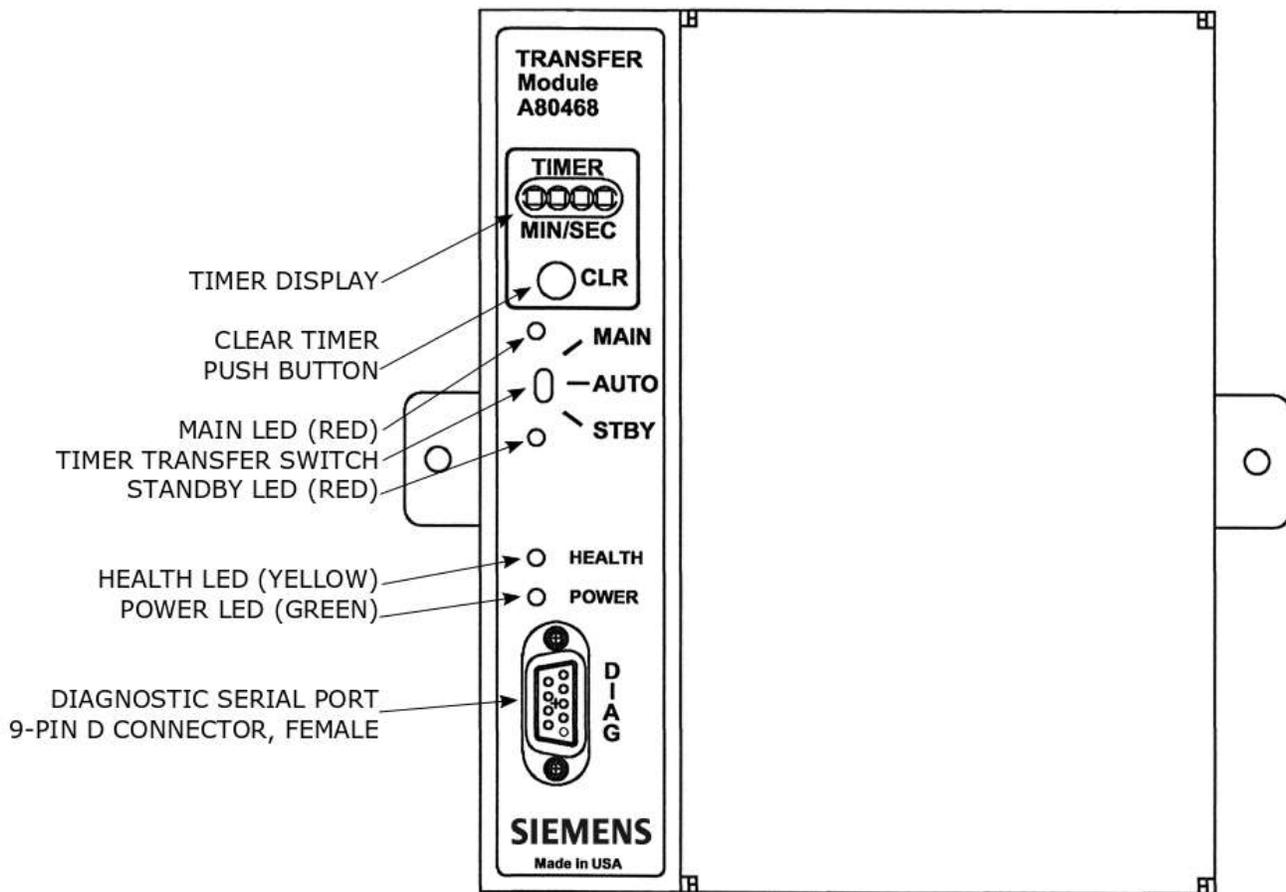
Figure 7-9 Transfer Assembly Front Panel
