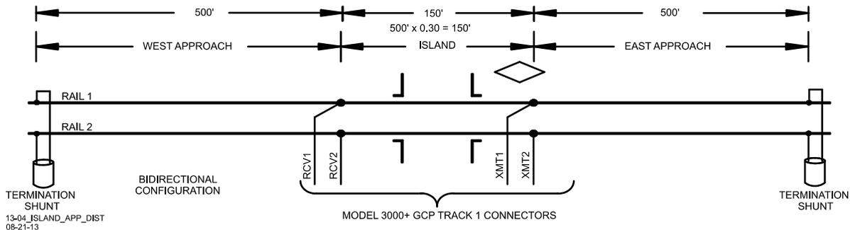
**Figure 2-10 Determining Island Approach Length**
