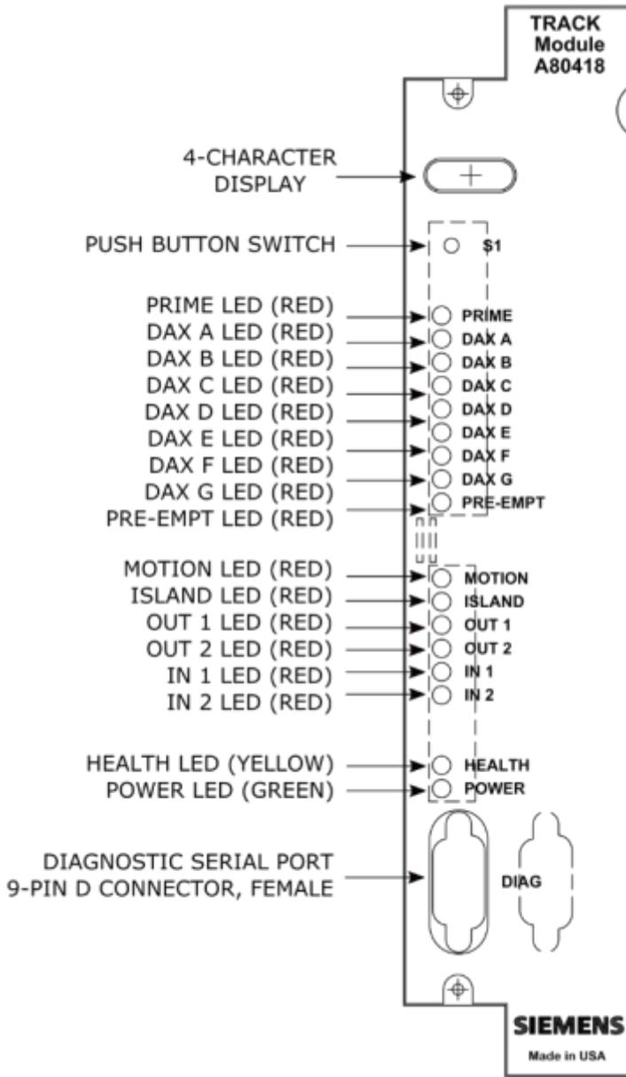
Figure 7-6 Track Module Front Panel
