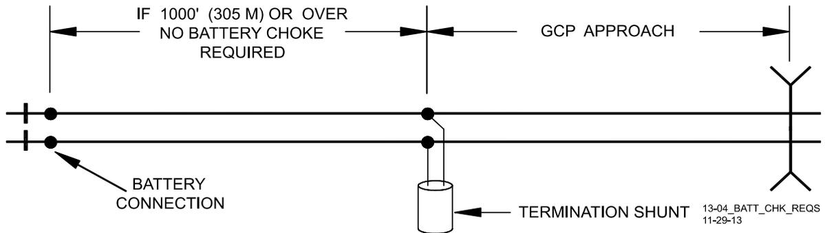
**Figure 6-19 Battery Choke Requirements**
