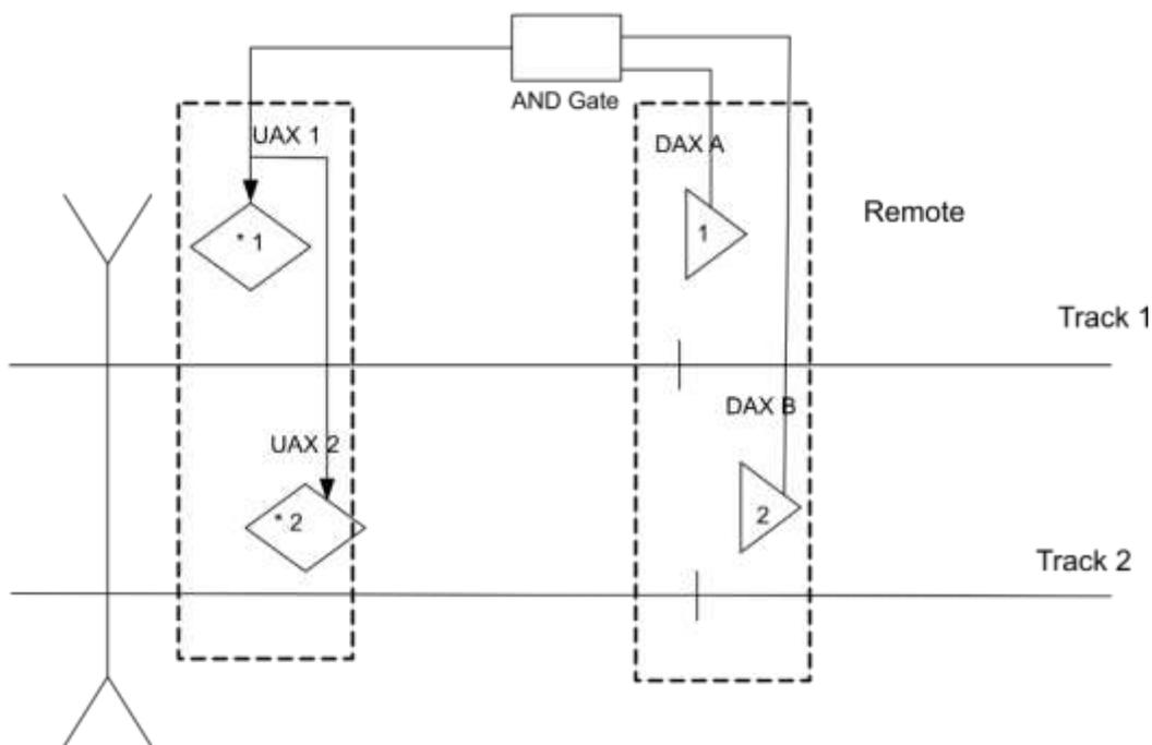
Figure 5-11 Double Track Single Wire Pair DAX / UAX
