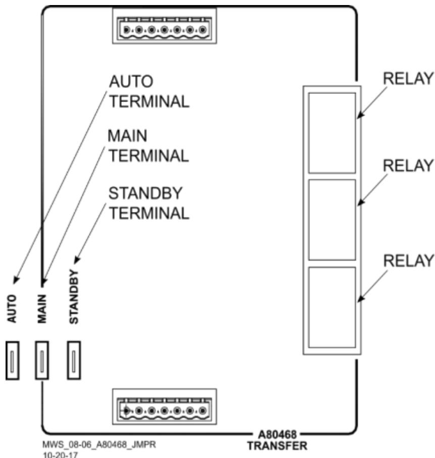
Figure 7-11 Transfer Module (A80468) Fuse Positions
