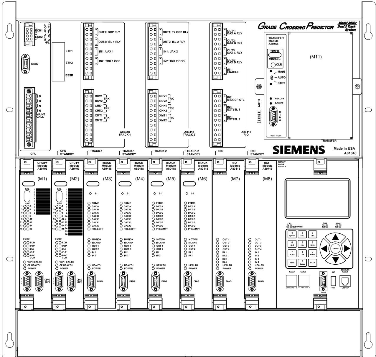
Figure 7-3 A81040 Case with Modules Installed
