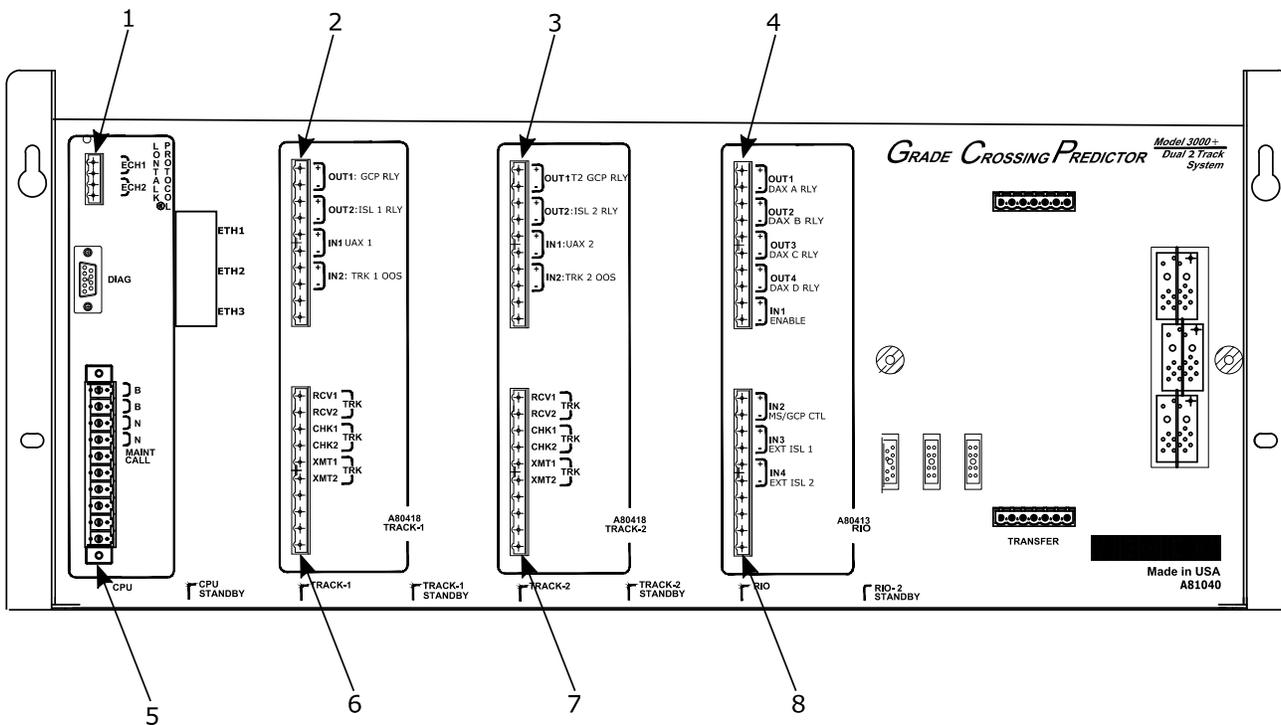
**Figure 7-4 External Wiring Connectors**
