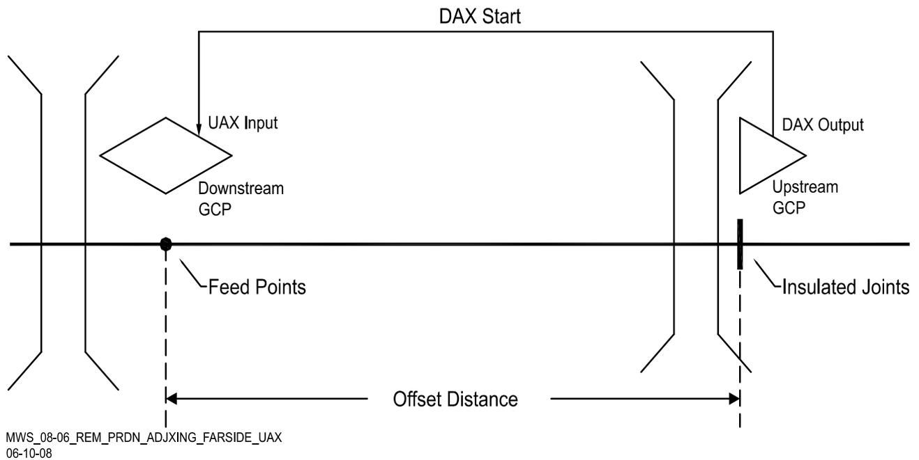
**Figure 5-2 Remote Prediction from an Upstream Crossing - Joints on Far**
