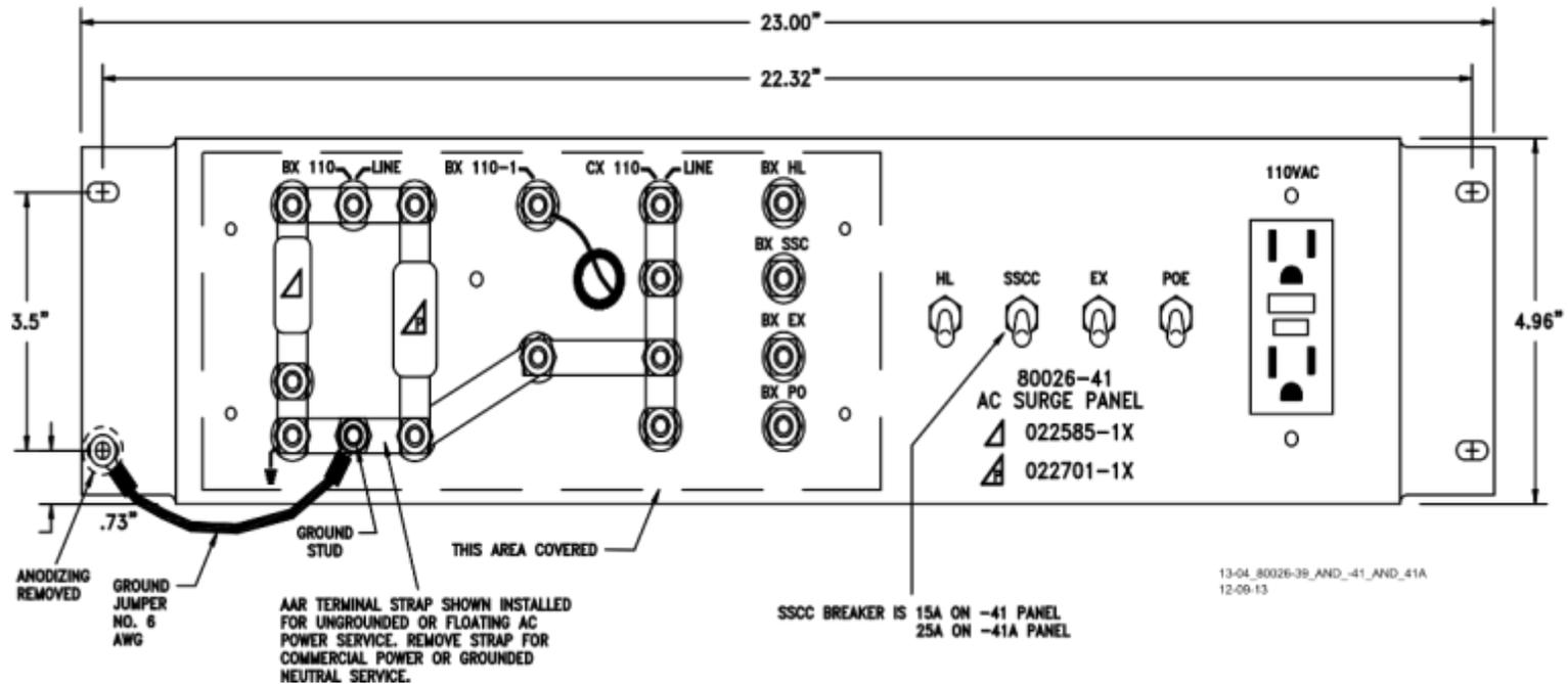
Figure 6-38 Rack Mounted Surge Panels, 80026-39, -41 and -41A
