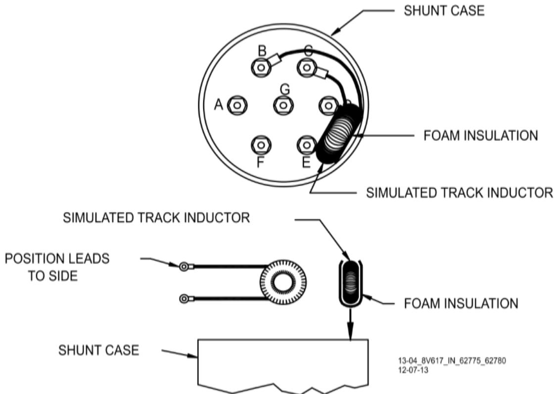
**Figure 6-15 Typical Installation of 8V617 in 62775/62780 Shunt**
