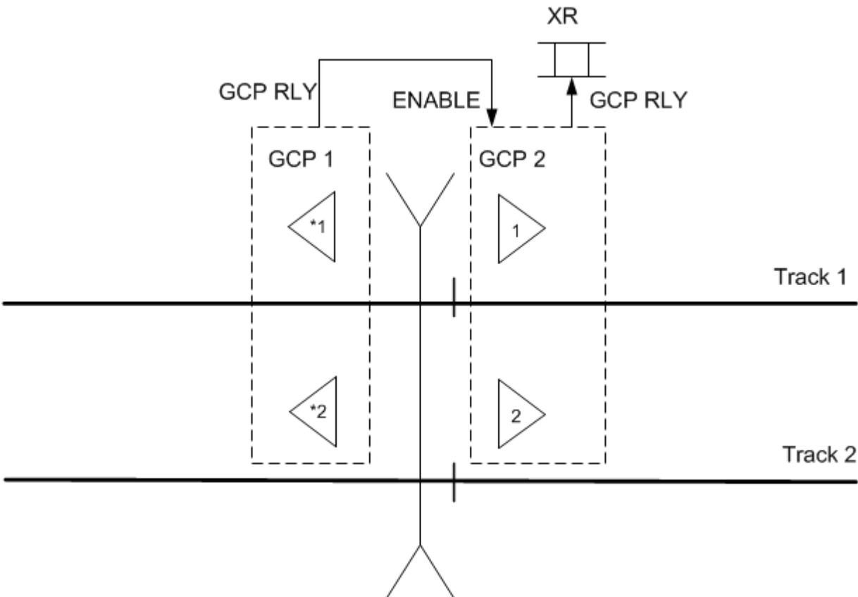
Figure 5-18 Double Track Installation with Back-to-Back GCP Units
