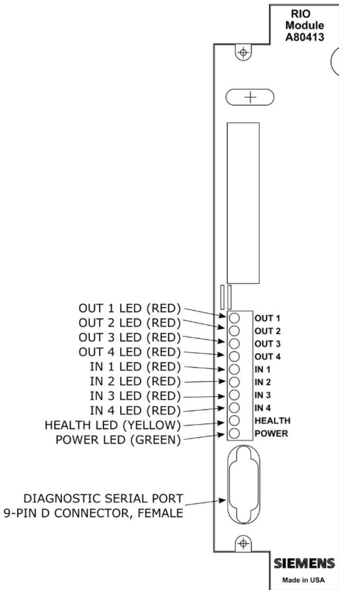
Figure 7-7 RIO Module Front Panel
