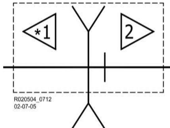
**Figure 5-22 Back-to-Back Unidirectional GCP Pair at a Crossing**
