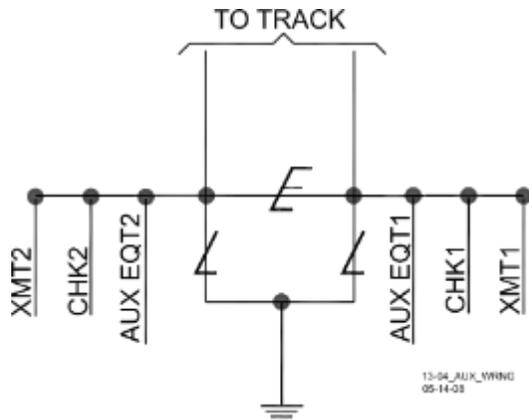
**Figure 2-13 Proper Connection of Track Leads**
