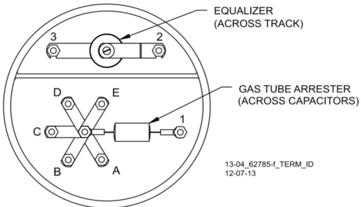
**Figure 6-29 Terminal Identification, 62785-f Tunable Insulated joint Coupler**
