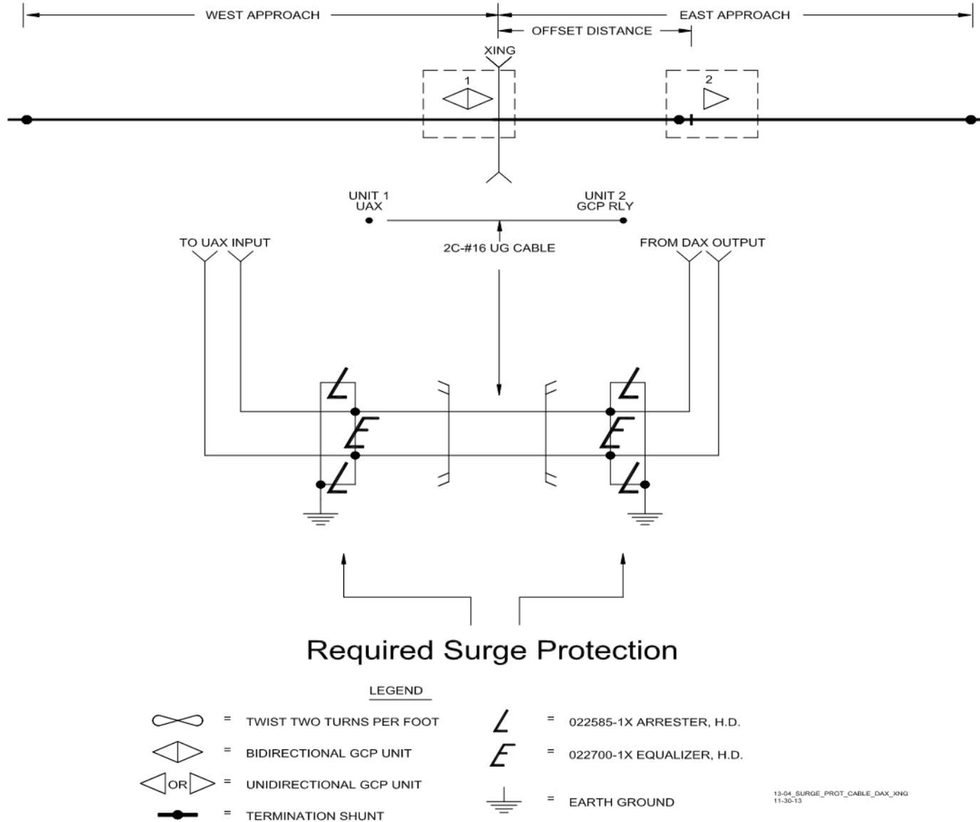
**Figure 2-32 Typical Surge Protection Requirements When Cabling Between Remote DAX Unit and Crossing Unit**
