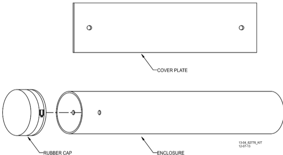
**Figure 6-31 MS/GCP Termination Shunt Burial Kit, 62776**
