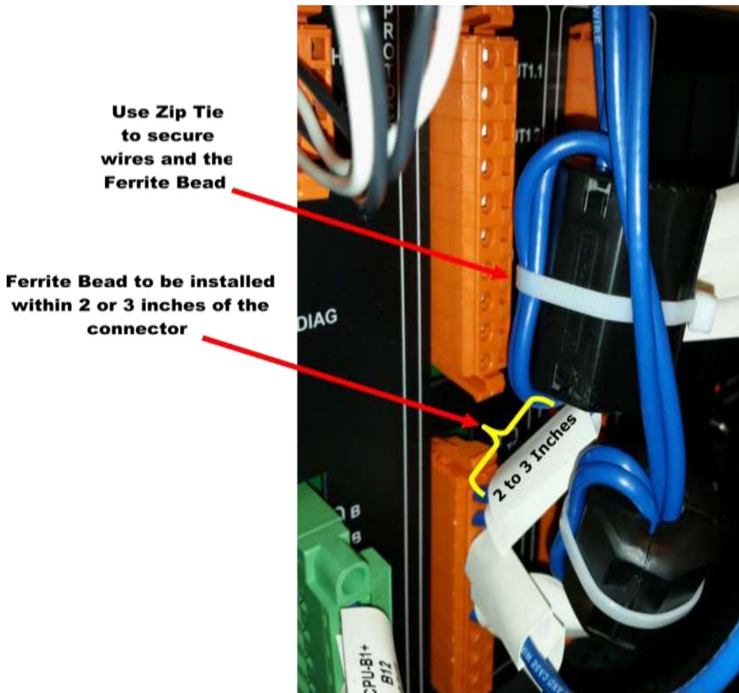
Figure B-15 Ferrite Bead Installation Guide
