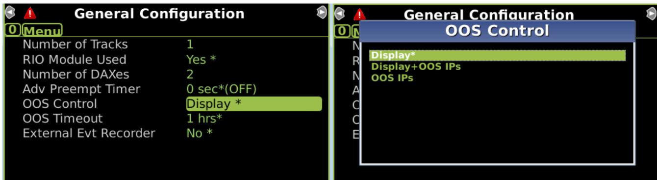
Figure 5-36 Out Of Service Display Settings
