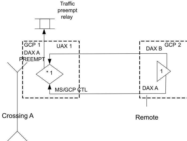
Figure 5-45 Remote Preemption from Separate Model 3000+ GCP Case
