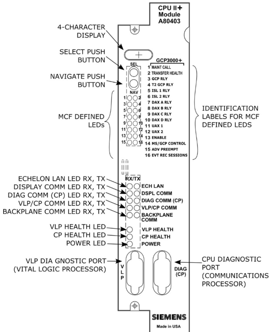
Figure 7-5 CPU II+ Front Panel
