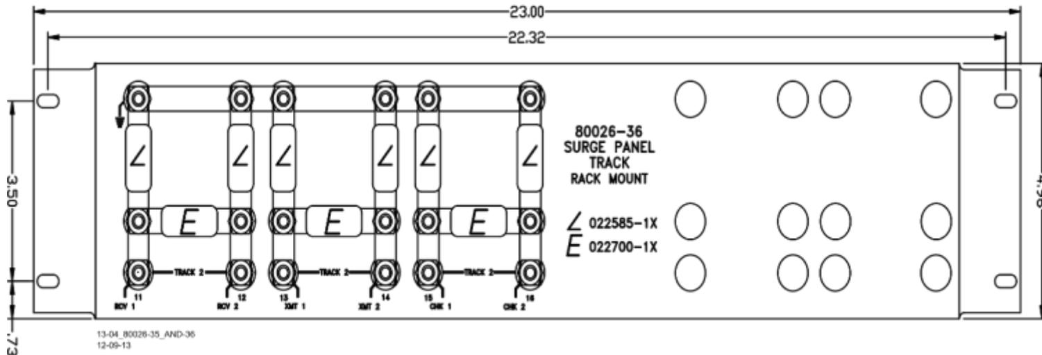
Figure 6-36 Rack Mounted Surge Panels, 80026-35 and -36
