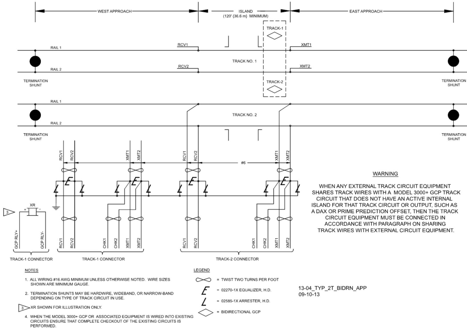
Figure 2-21 Typical Two Track Bidirectional Application
