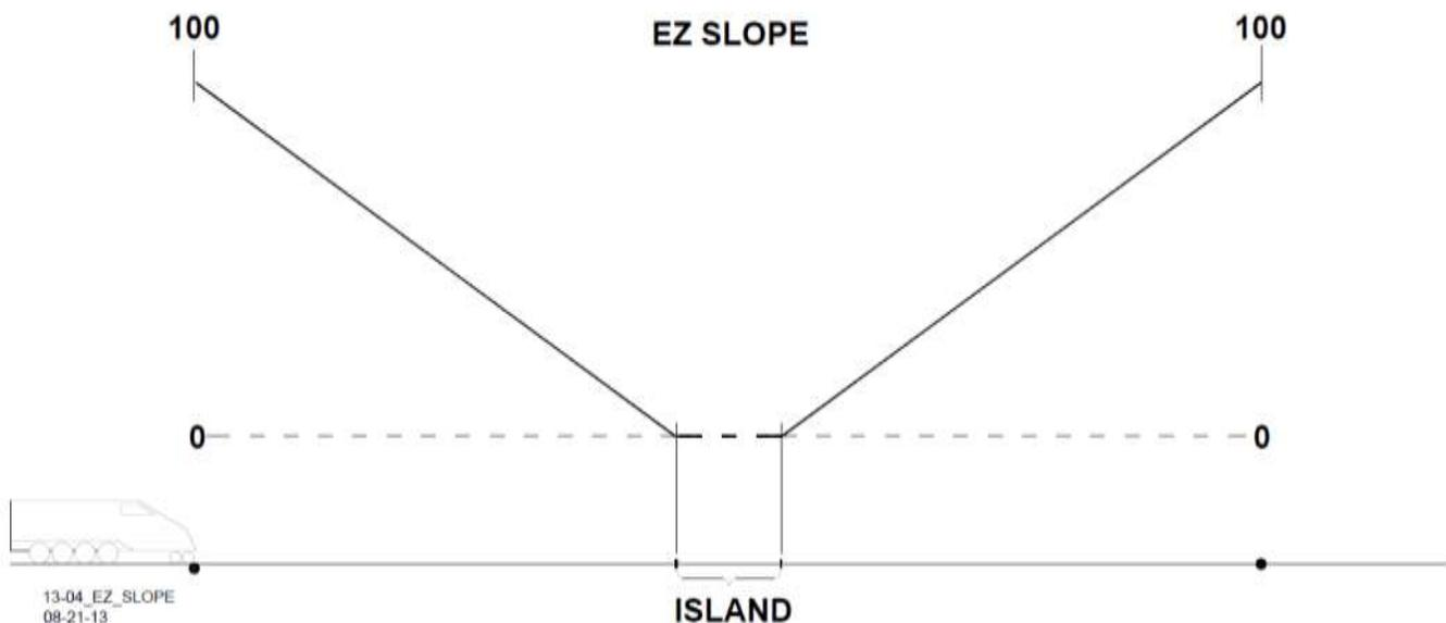
**Figure 1-1 Diagram of EZ Level Compared to Train Shunt Location**
