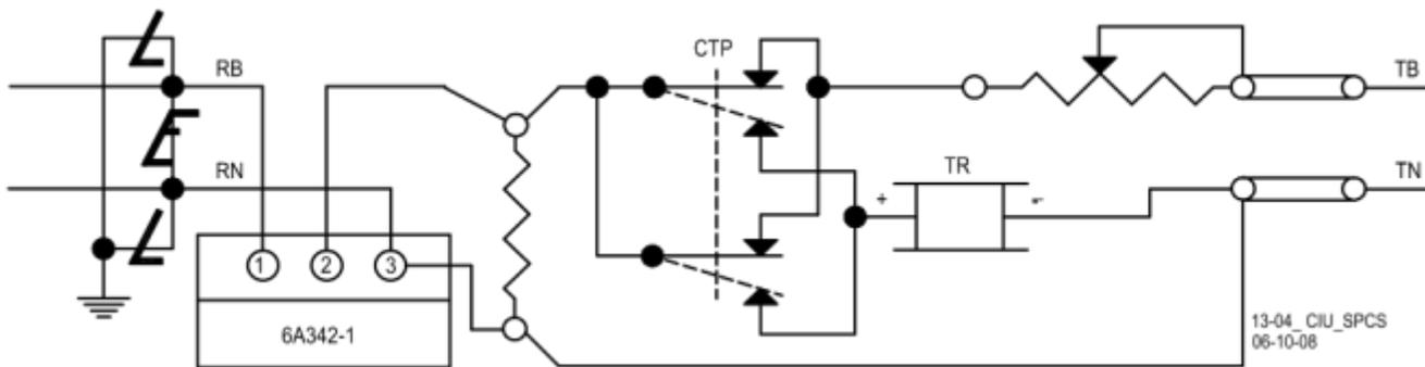
**Figure 6-23 Code Isolation Unit in a Single Polarity Code System**
