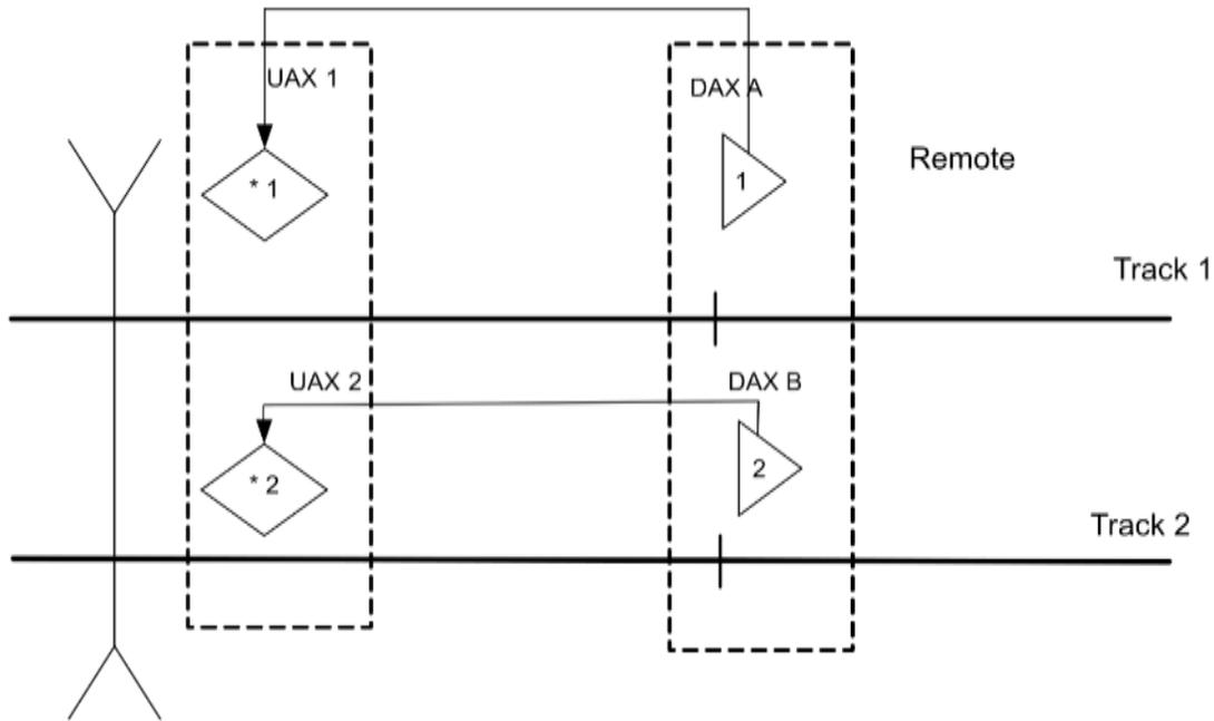
Figure 5-14 Double Track with Independent UAXes
