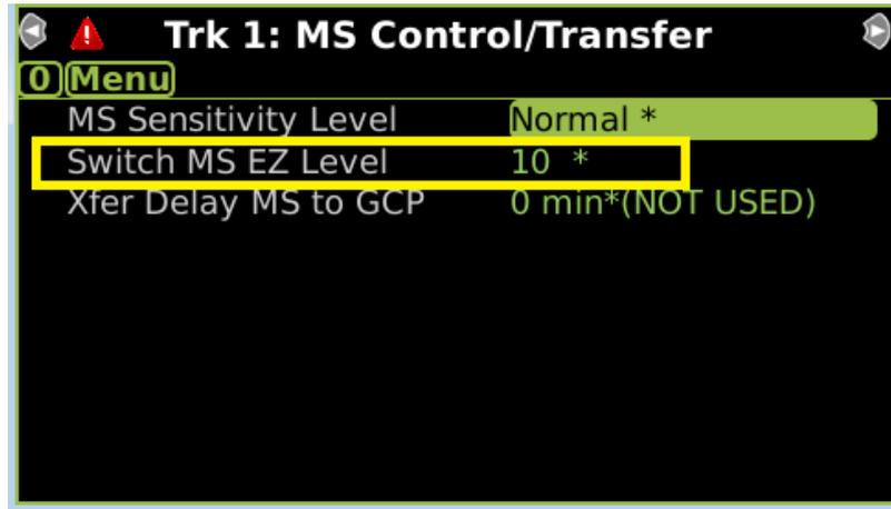
Figure 5-26 Switching from Predictor to Motion Sensor Operation
