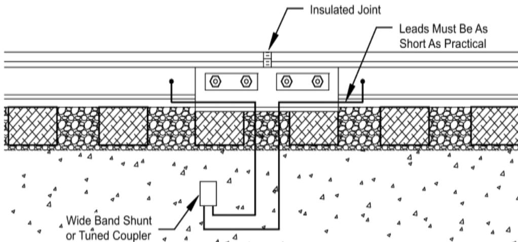
**Figure 2-9 Insulated Joint, Shunt, or Coupler Installation**
