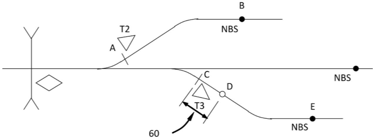
Figure 5-7 T2 or T3 Less than 1000 Ft
