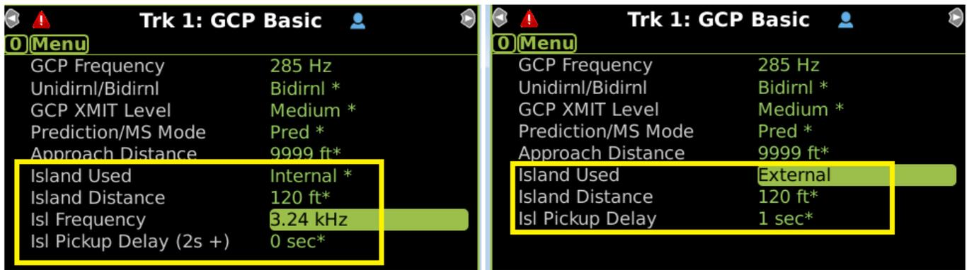
Figure 5-23 Internal Island Pickup Delay
