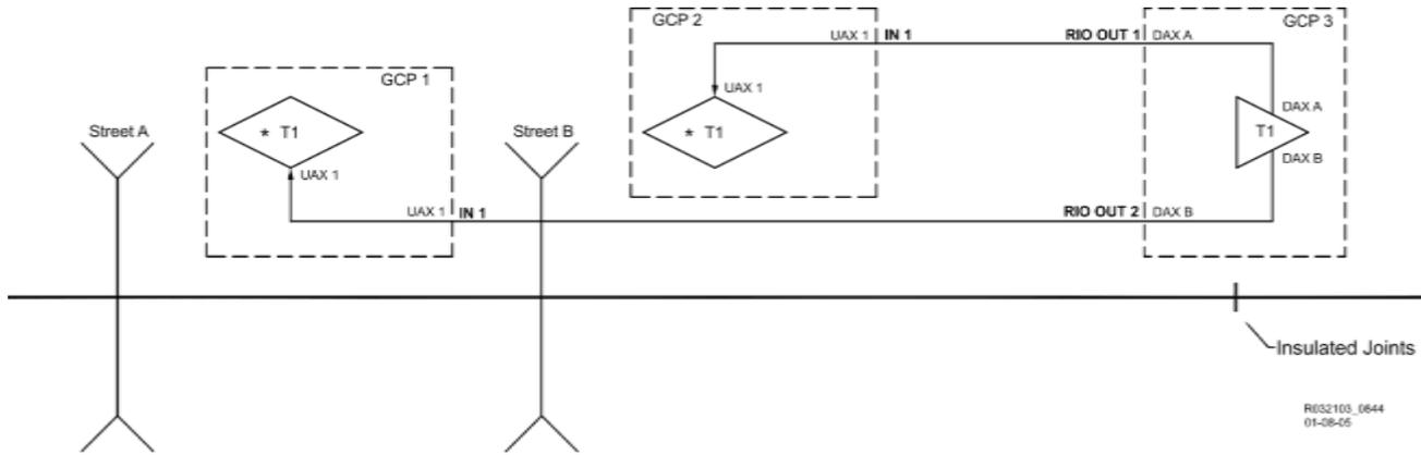
Figure 5-15 Remote Prediction for Multiple Bidirectional Crossings
