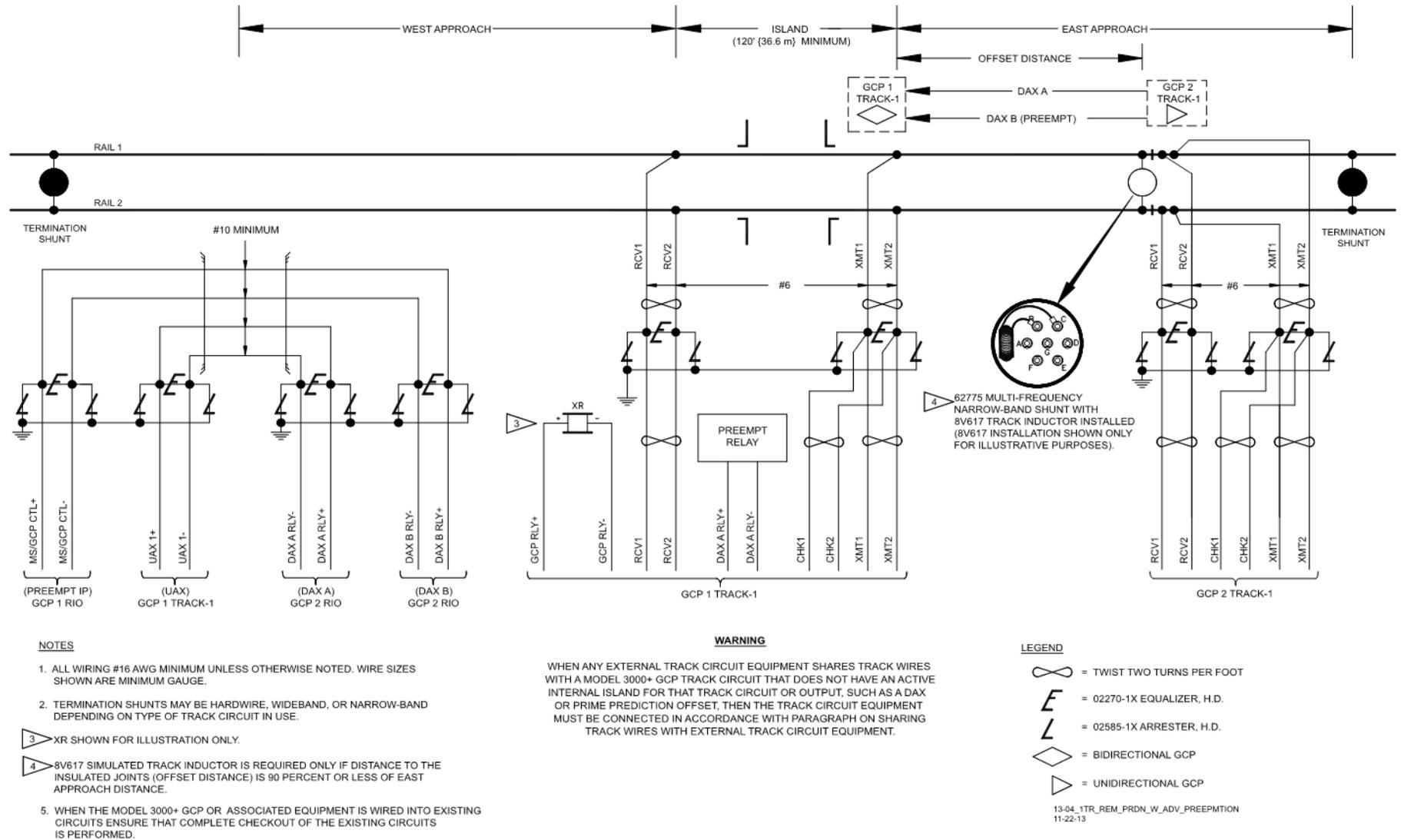
Figure 2-29 Single Track, Remote Prediction with Advanced Preemption
