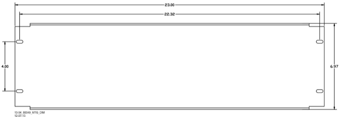
Figure 6-6 DC Shunting Enhancer Panel Mounting Dimensions
