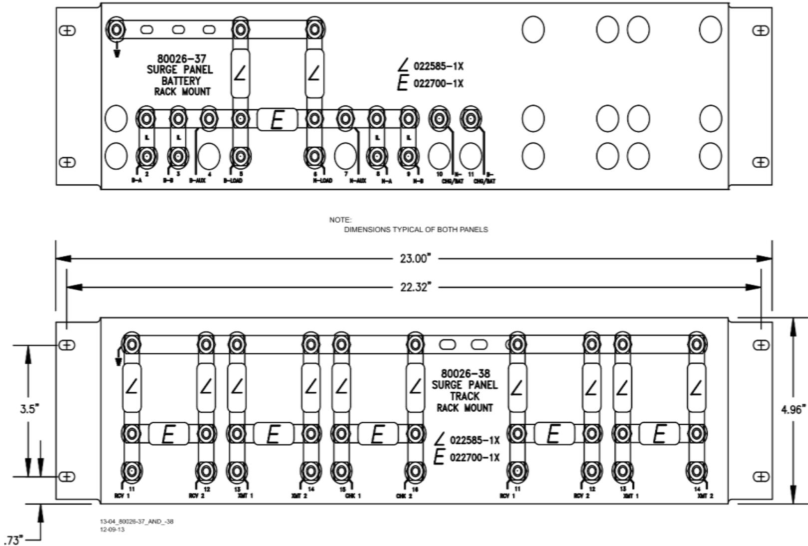
Figure 6-37 Rack Mounted Surge Panels, 80026-37 and -38
