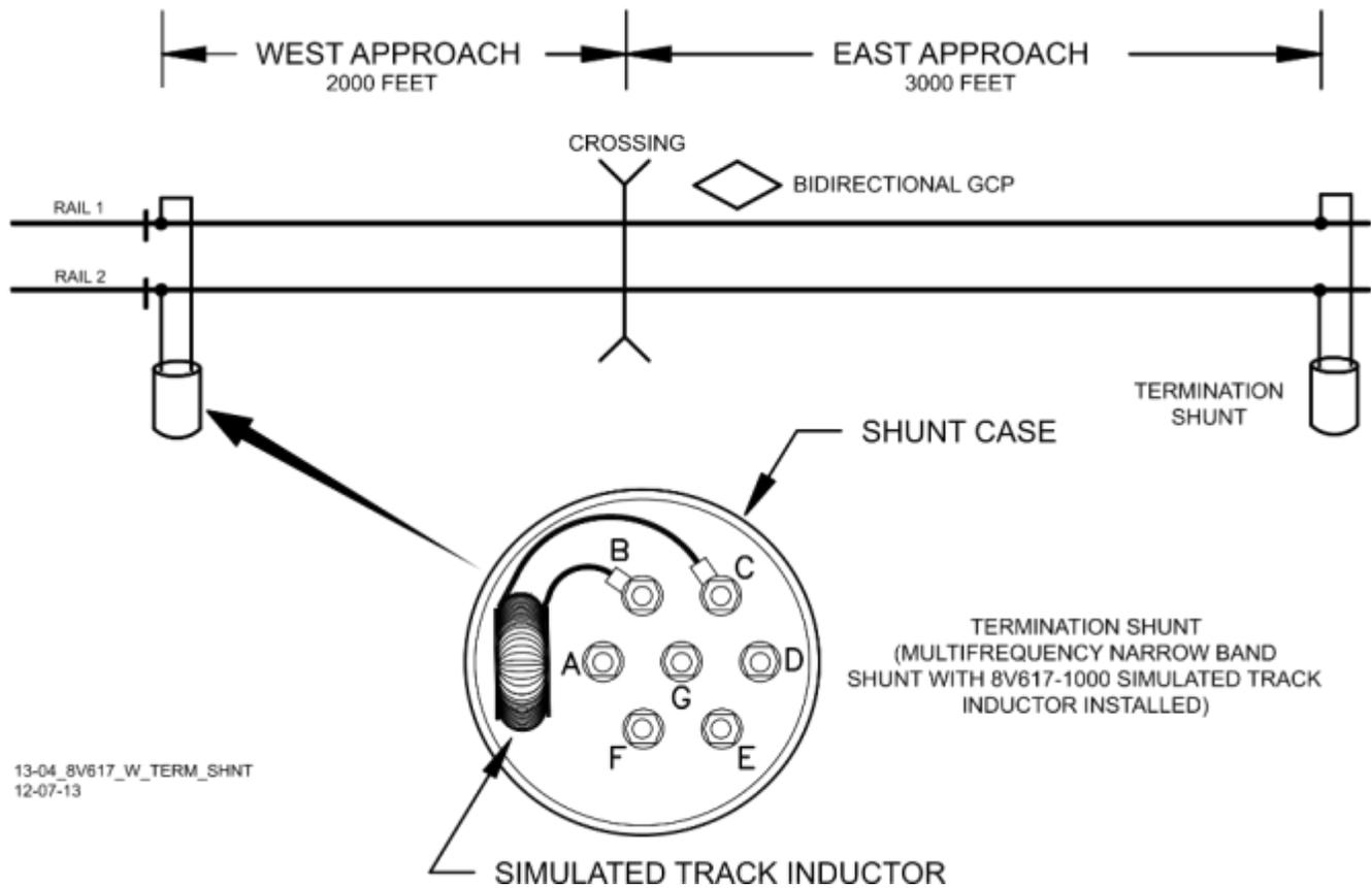
Figure 6-14 Simulated Track Inductor Used with Termination Shunt
