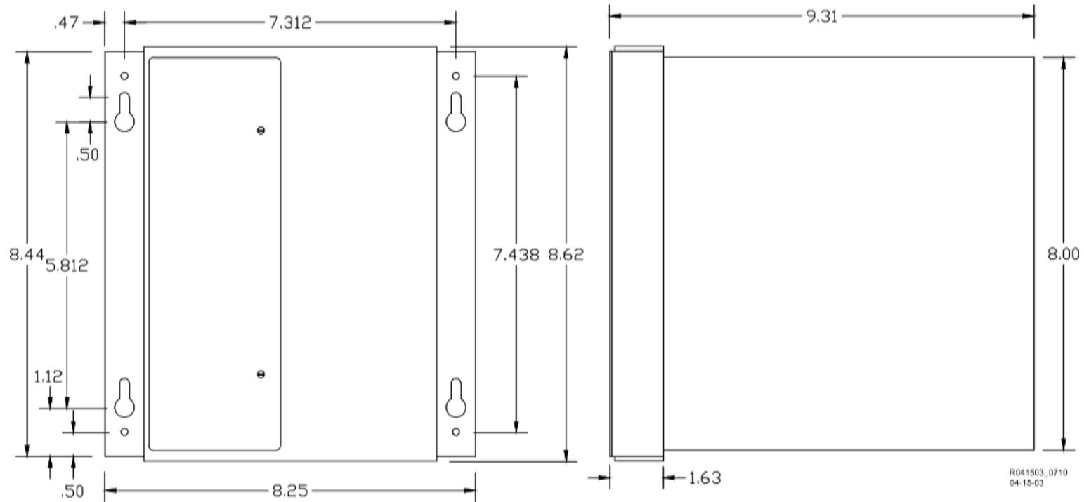
**Figure 6-3 Bidirectional Simulation Coupler Assembly Mounting Dimensions**
