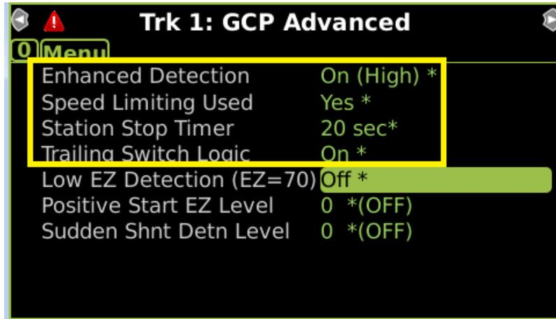
Figure 5-35 Poor Shunting Logic Parameters
