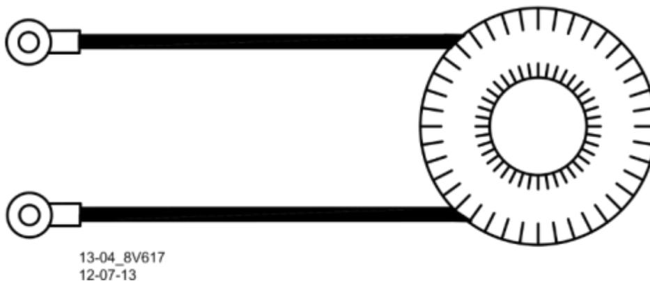
**Figure 6-13 Simulated Track Inductor, 8V617**
