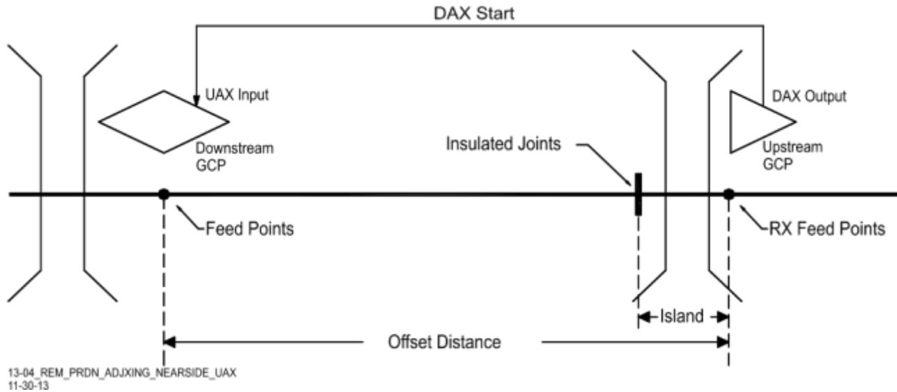
Figure 5-3 Remote Prediction from an Upstream Crossing - Joints on Near Side
