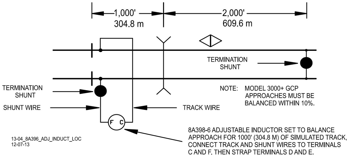
**Figure 6-17 Adjustable Inductor Used with Termination Shunt**
