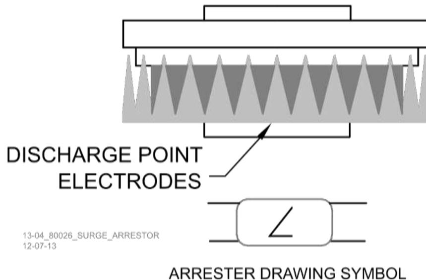
Figure 6-32 Typical 80026 Surge Panel Arrester Mounting Position
