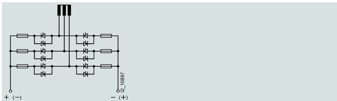
Six-pulse bridge circuit B6 with branch fuses (reversible connection)
