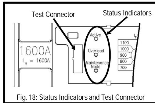
Fig. 18: Status Indicators and Test Connector
