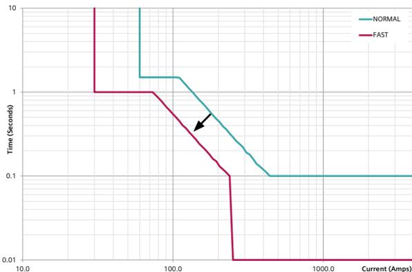
Fast curve  $i^2t$  is a configurable fraction of the normal curve  $i^2t$
