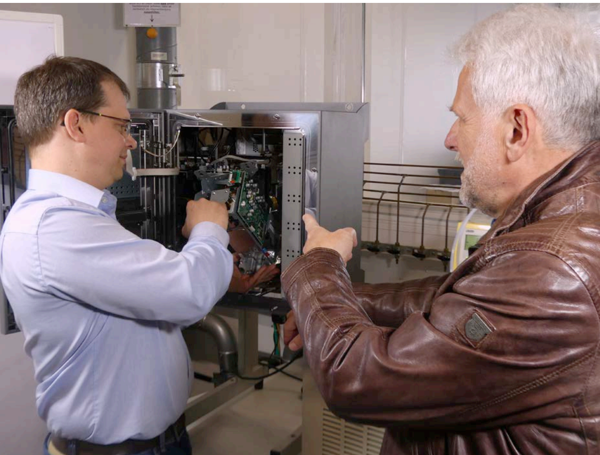
Quick and easy exchange of the modules thanks to the „Plug&Measure“ feature.
