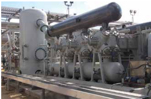
HOSS compressor for a CO 2 application.
